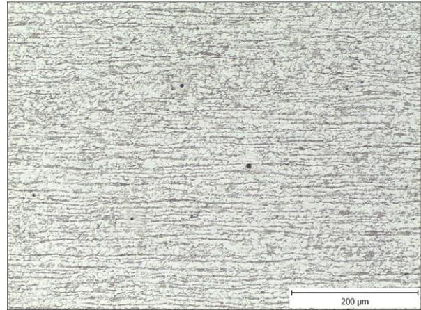
**Fig. 4 The microstructure in base metal**
