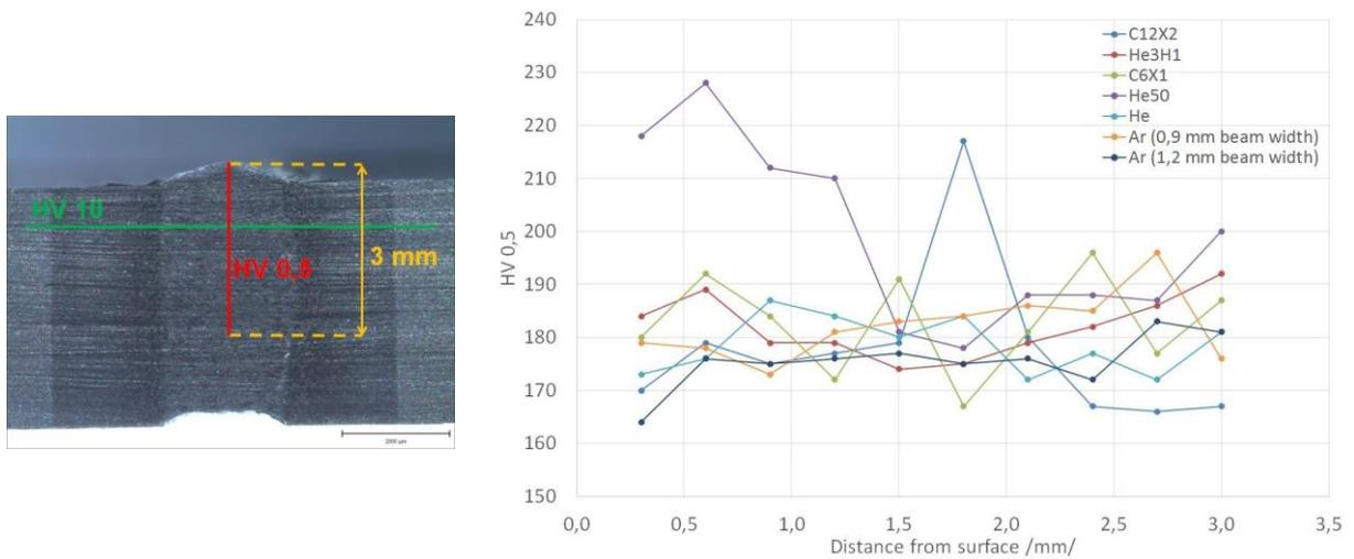
**Fig. 5 and 6 Summary of microhardness HV0,5 profile measurement**
