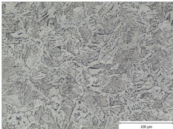
Fig. 1 The microstructure in weld metal
