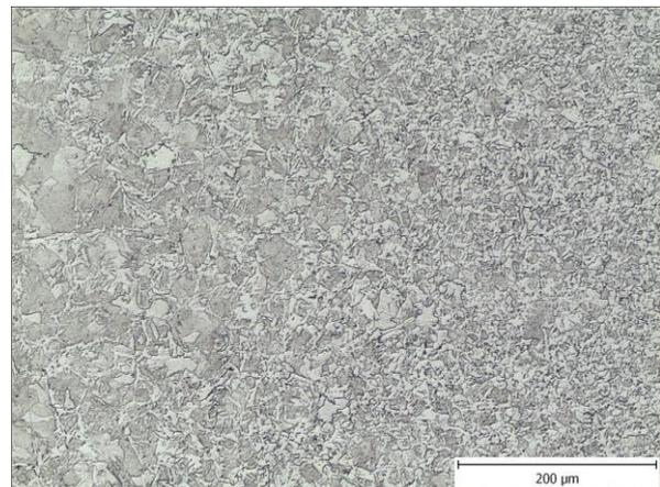
Fig. 2 The microstructure at weld metal-HAZ borderline
