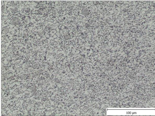
**Fig. 3 The microstructure in HAZ**
