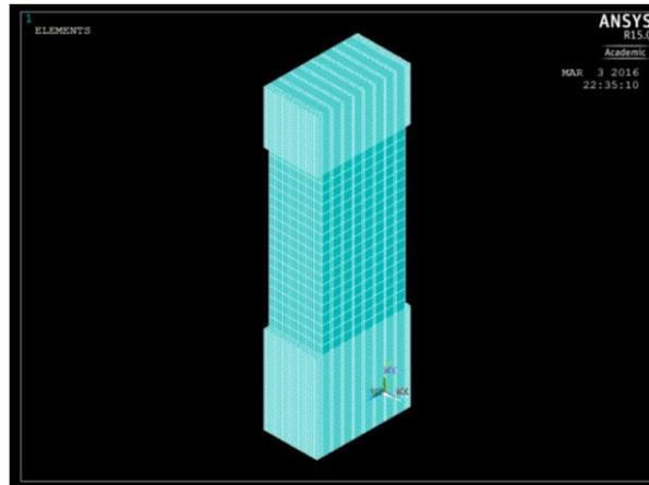
Fig. 6: Simulation of spring package with screen based on ANSYS FEM-element “solid185.
