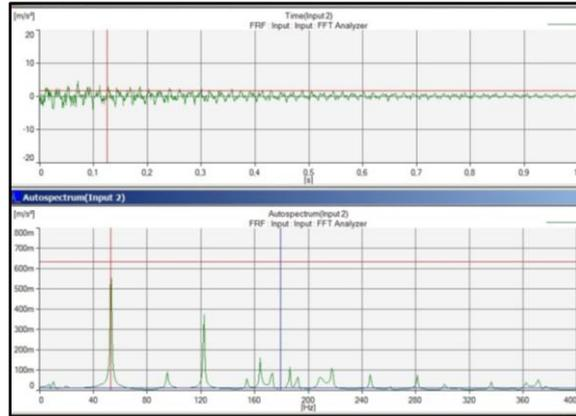
Fig. 4: Result of tangential excitation in vertical direction (own source).
