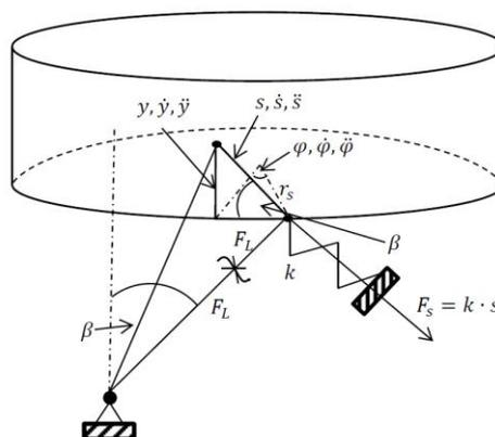
Fig. 5: Motion model of the fix point of the conveying element.
