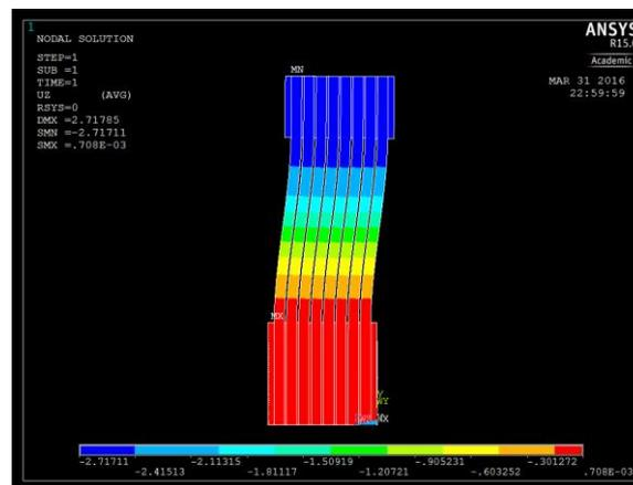
Fig. 7: Displacement in z-direction.
