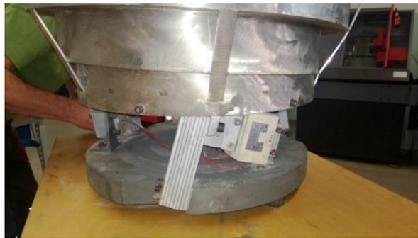
Fig. 3: Spring package with excitation device 220/230 V, 25Hz.
