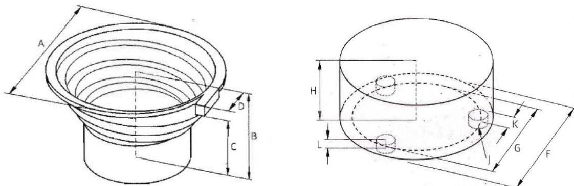
Fig. 2: Parameters Sortimat bowl feeder type SMB 6 (own source).
