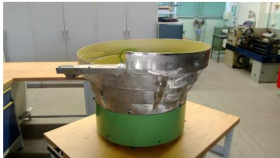
Fig. 1: Sortimat bowl feeder type SMB 6 (own source).
