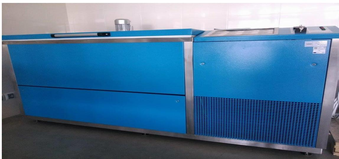
Fig. 1: The equipment for testing freeze – thaw resistance
