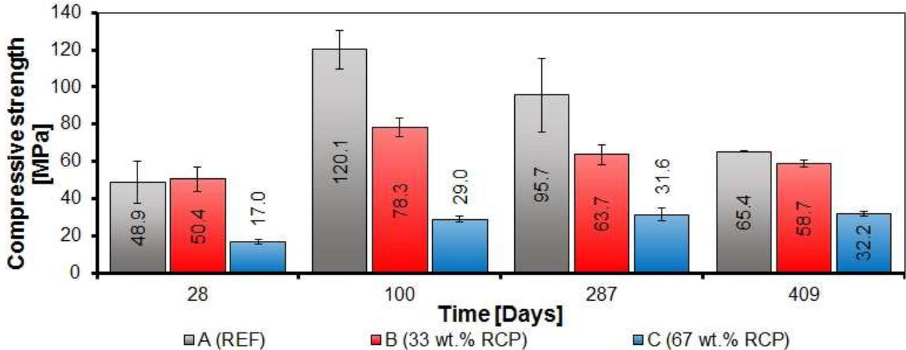
Fig. 2: Compressive strength development of cement pastes with different amount of a recycled concrete powder.
