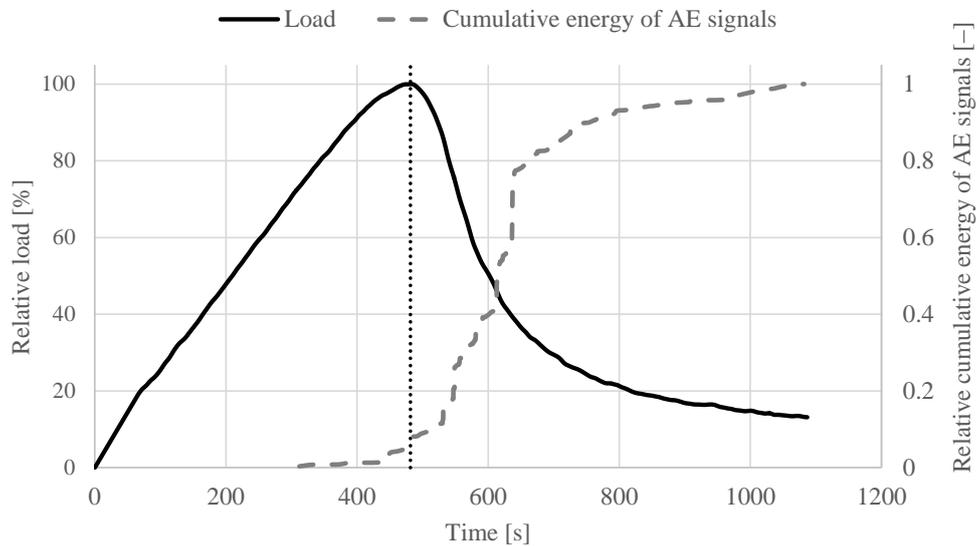
Fig. 3: Dependence of relative cumulative energy of AE signal and the relative load on time. (REF sample)
