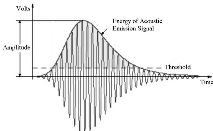
Fig. 1: Typical AE signal
