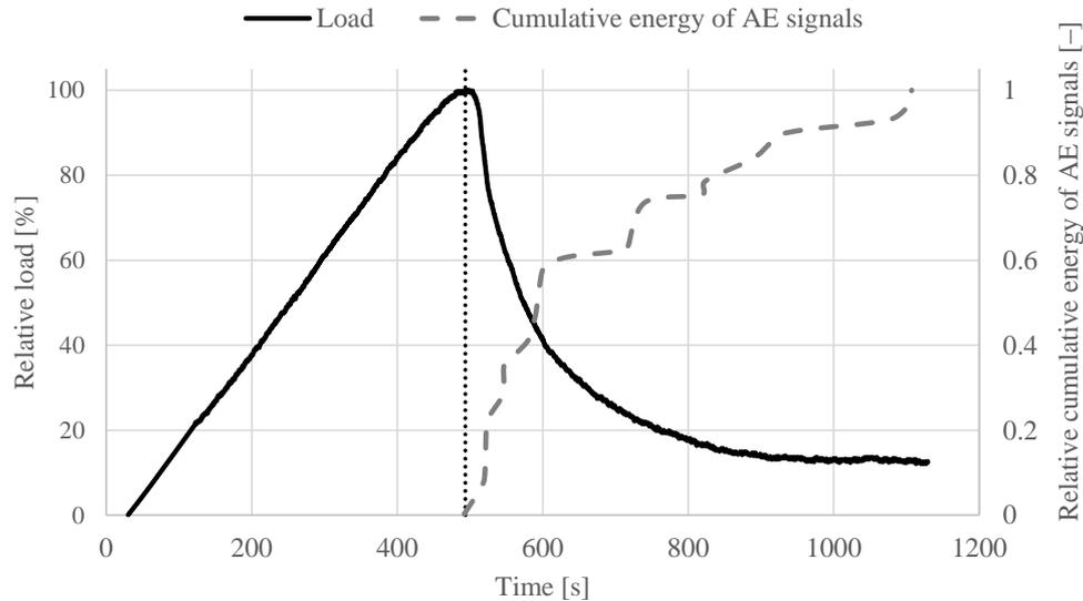
Fig. 4: Dependence of relative cumulative energy of AE signal and the relative load on time. (COND 10 sample)
