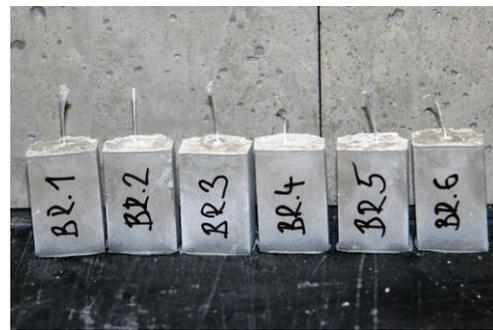
Fig. 2: Cement samples prepared for single-fiber pull out tests.
