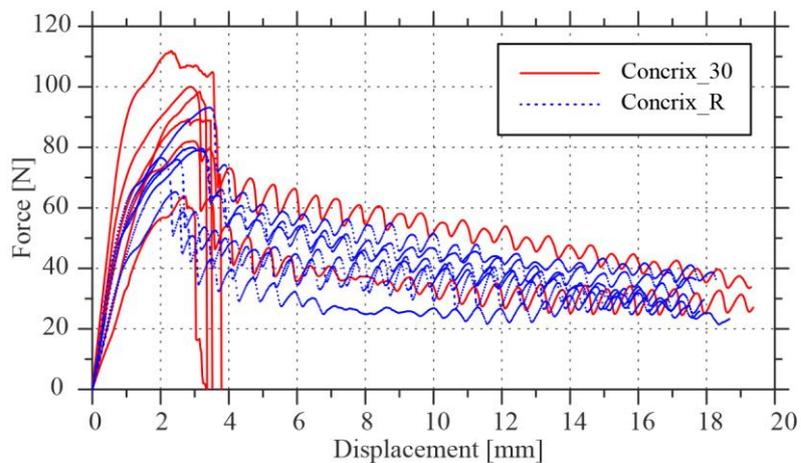
Fig. 5: Loading force depending on fiber free-end displacement obtained during pull out testing.
