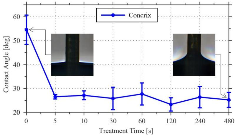
Fig. 3: Contact angle sizes depending on plasma treatment time obtained during contact angles measurements.
