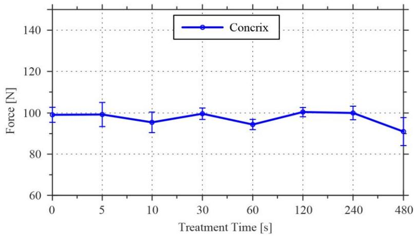
Fig. 4: Force needed to break the fibers depending on treatment time.
