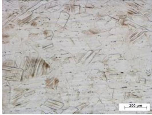
Fig. 1: Microstructure of AISI 316L
