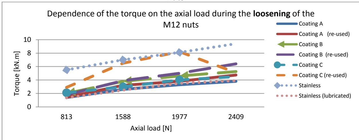
**Fig. 6.** Dependence of the torque on the axial load during the **loosening** of the M12 nuts.
