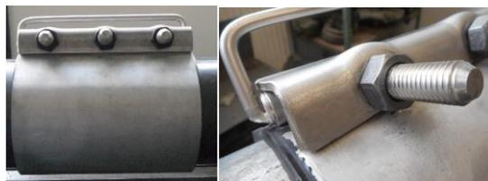
**Fig. 1.** Example of a repair clamp and the tightening screwed joint - Laboratories of the Faculty of Mechanical Engineering CTU in Prague.
