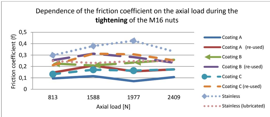
**Fig. 7.** Dependence of the friction coefficient on the axial load during the **tightening** of the M16 nuts.
