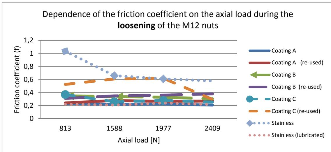
**Fig. 10.** Dependence of the friction coefficient on the axial load during the **loosening** of the M12 nuts.
