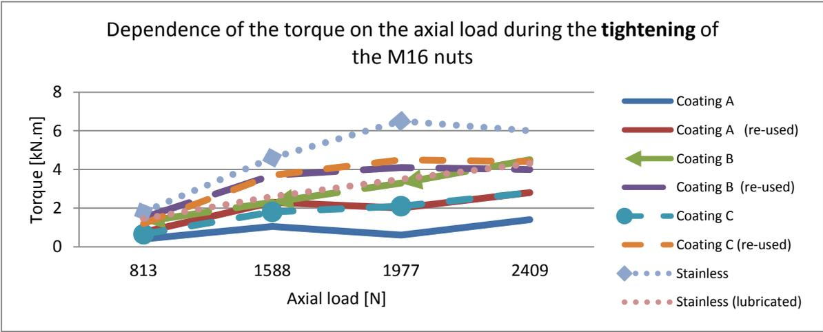
Fig. 3. Dependence of the torque on the axial load during the tightening of the M16 nuts.
