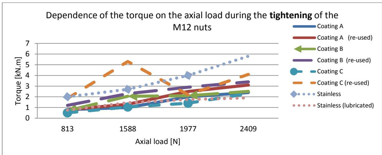
**Fig. 5.** Dependence of the torque on the axial load during the **tightening** of the M12 nuts.
