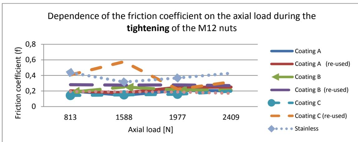
**Fig. 9.** Dependence of the friction coefficient on the axial force during the **tightening** of the M12 nuts.
