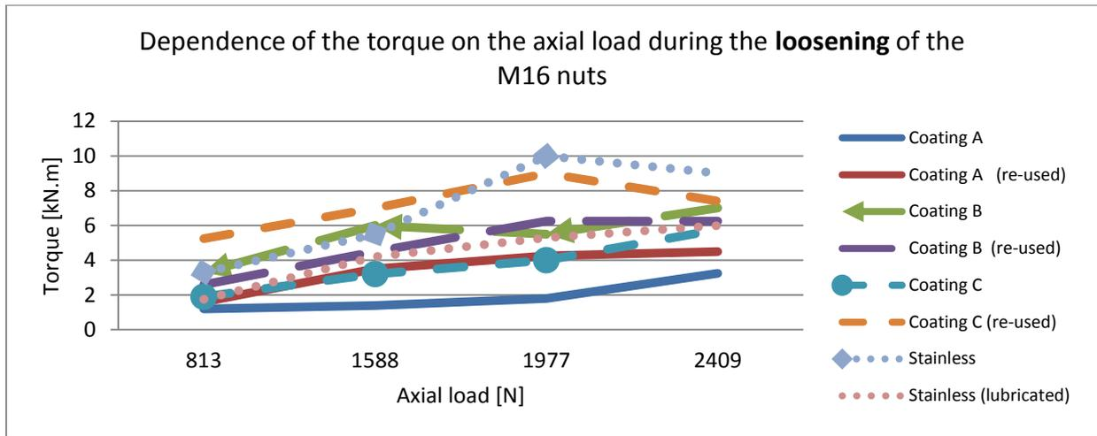
**Fig. 4.** Dependence of the torque on the axial load during the **loosening** of the M16 nuts.
