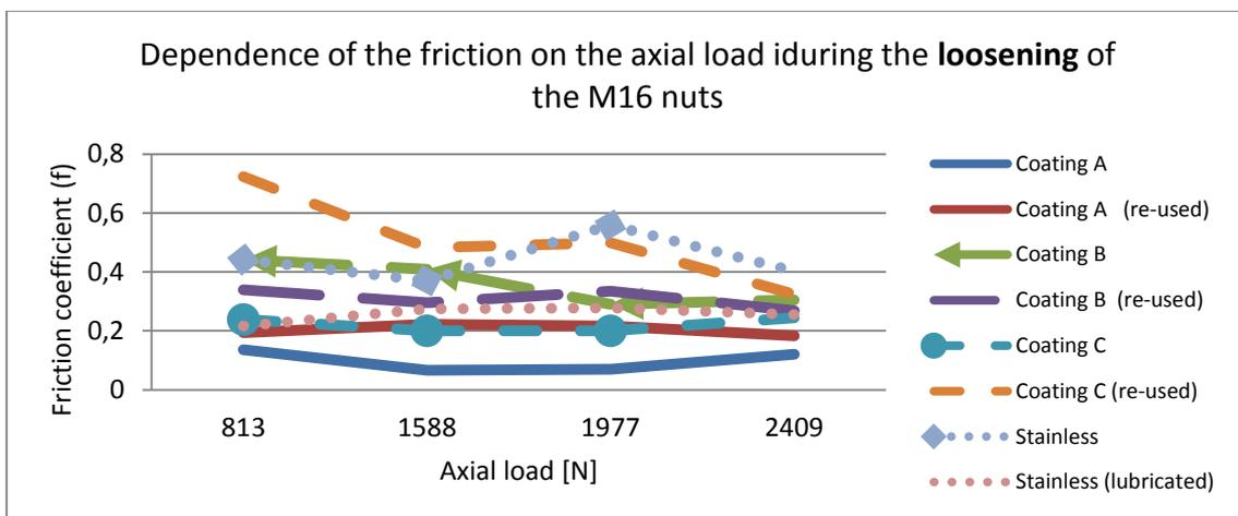
**Fig. 8.** Dependence of the friction coefficient on the axial load during the **loosening** of the M16 nuts.
