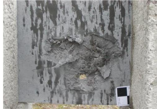
Fig. 9 4-cm slab – back side – craters after .7,62x39 mm soft core caliber (two upper did not go through, lower did).
