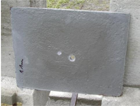
Fig. 2 1-cm slab – .22 caliber on the left, 9 mm Luger caliber on the right side of the slab.
