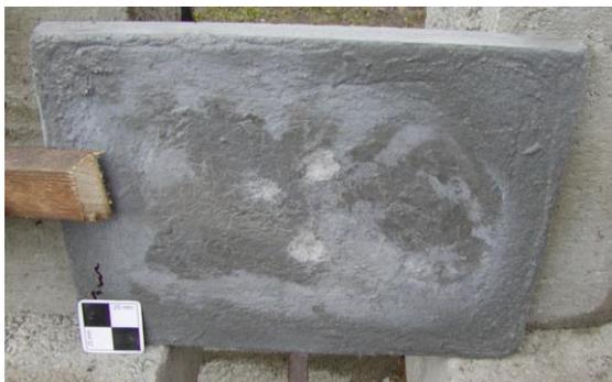
Fig. 6 3-cm slab – hit from 9 mm Luger caliber on the left and two hits from 62x25 mm Tokarev caliber on the right side.
