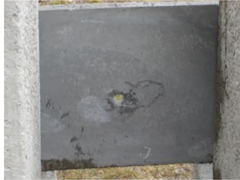
Fig. 3 1-cm slab – back side – crater after 9 mm Luger on the left and crater after .22 caliber on the right side of the slab.
