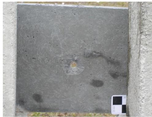
Fig. 5 2-cm slab – back side – nothing visible from .22 caliber and bullet hole from 9 mm Luger caliber.
