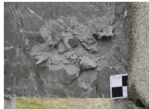
Fig. 11 5-cm slab – back side – craters after .7,62x39 mm steel core caliber (two upper did not go through, lower did).
