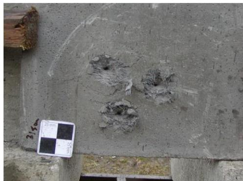
Fig. 10 5-cm slab – craters after .7,62x39 mm steel core caliber (two upper did not go through, lower did).
