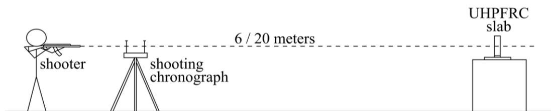
Fig. 1 Schema of the applied shooting system.
