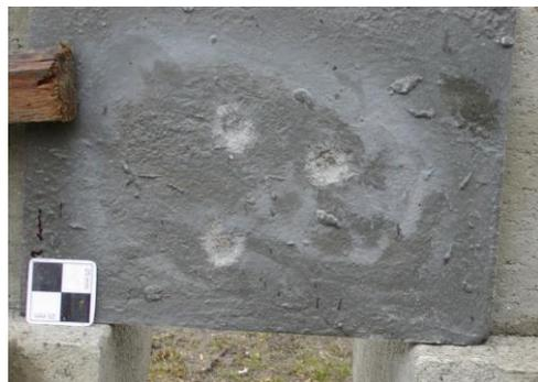
Fig. 7 3-cm slab – three hits from .44 Magnum caliber.
