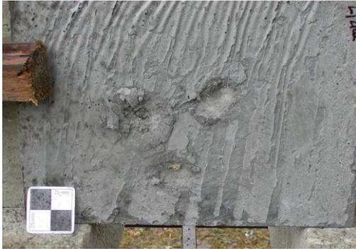
Fig. 8 4-cm slab – craters after .7,62x39 mm soft core caliber (two upper did not go through, lower did).
