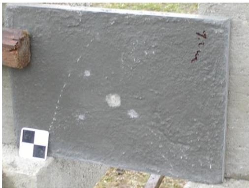
Fig. 4 2-cm slab – three small craters are from .22 caliber, one bullet hole in the middle is from 9 mm Luger caliber.
