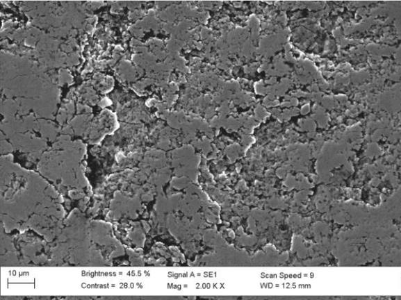
Fig. 1 Example of surface fretting fatigue damage of axle seat under press fit with microcracks and short fatigue cracks
