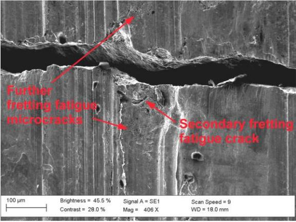
Fig. 2 Main fatigue crack under press fit with secondary crack and further fretting fatigue microcracks
