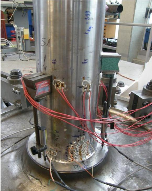
Fig. 4 LVDT extensometers measuring displacement between axle and wheel
