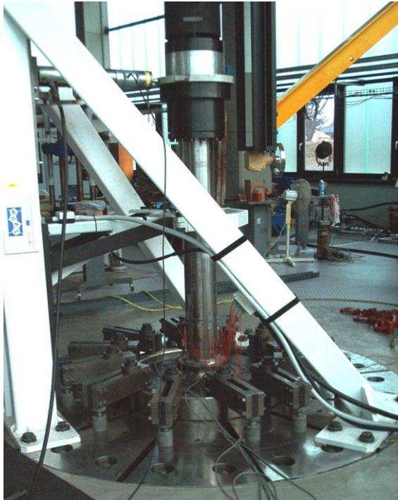
Fig. 3 Total view of the axle prepared for fatigue test on the Sincotec machine
