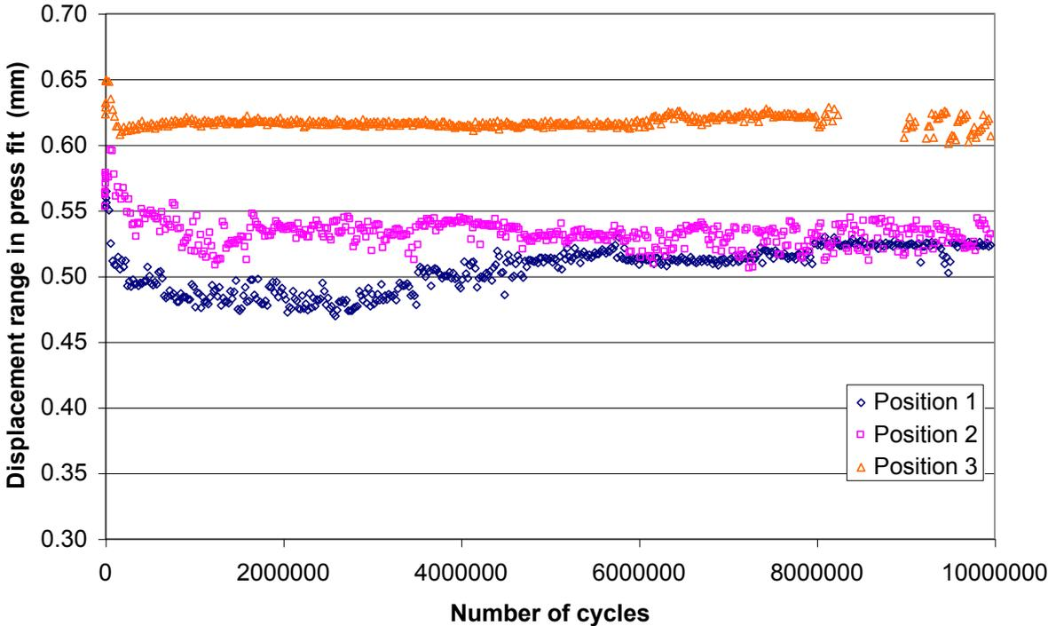
Fig. 5 Displacement range as measured by the extensometers at three circumferential points as dependence on number of fatigue load cycles
