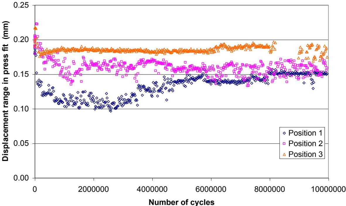
Fig. 6 Pure values of displacement between axle and hub during fatigue test after correction for elastic deformation of the part of the axle with magnetic holders
