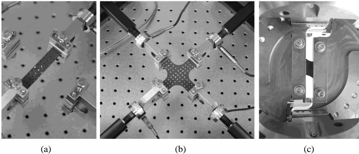
Fig. 2. Performed tests: uniaxial tension (a), biaxial tension (b), and shear of Arcan sample (c).
