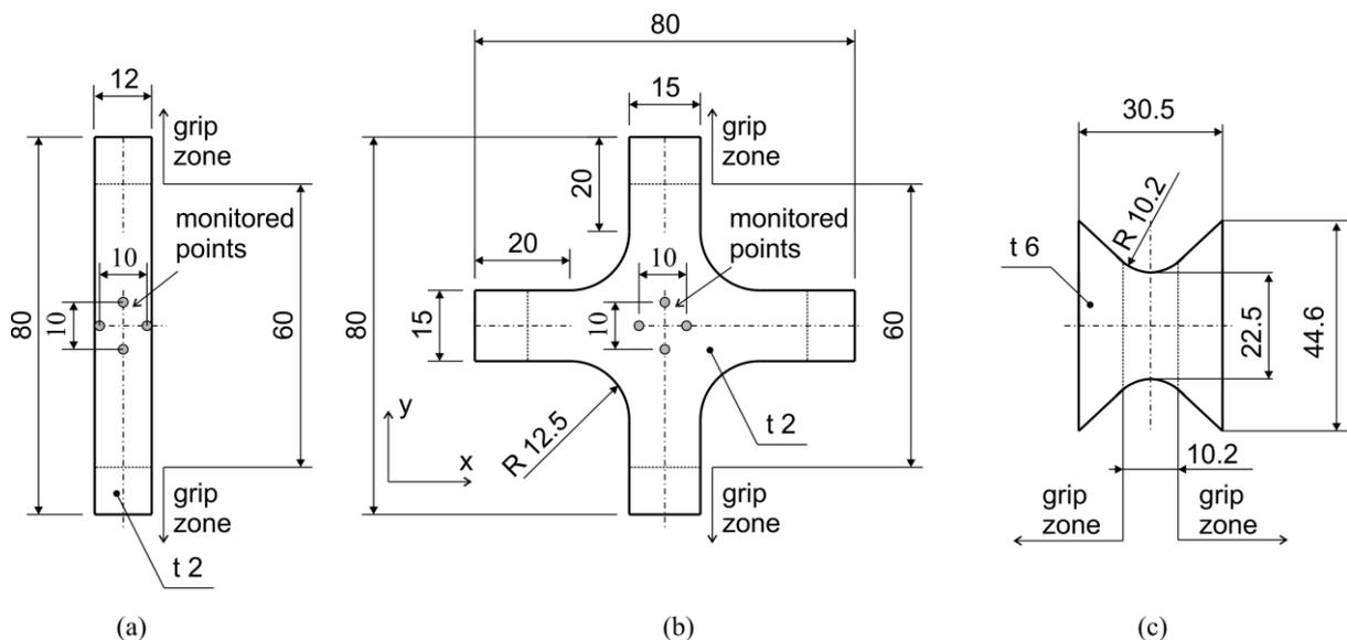
Fig. 3. Samples for: uniaxial tension (a), biaxial tension (b), and shear (c).
