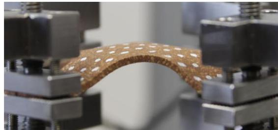
Fig. 8 Buckling of TB samples
