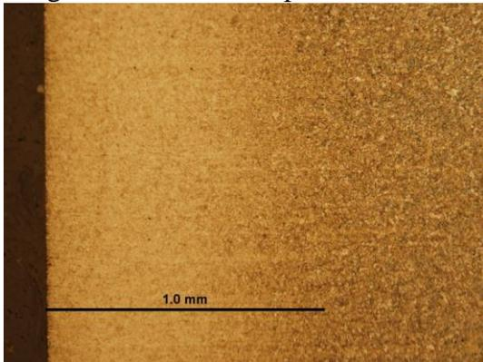
**Fig. 6** Depth of the carburized layer is about 0,8 mm
