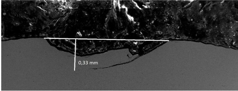
**Fig. 5** Depth of damage determining
