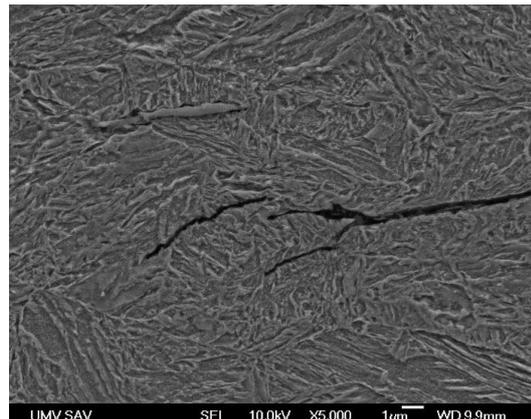
**Fig. 8** Detail of the crack root
