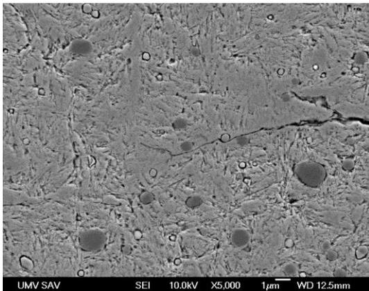
**Fig. 7** Crack root shown with carbides
