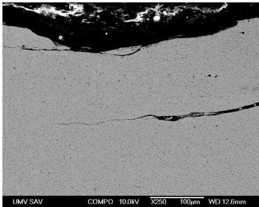
Fig. 3 Detail of the damaged part shown in regime COMPO
