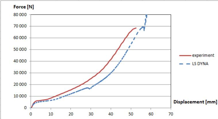
Figure 2: Comparison between numerically and experimentally found material behaviors (quasistatic compression)
