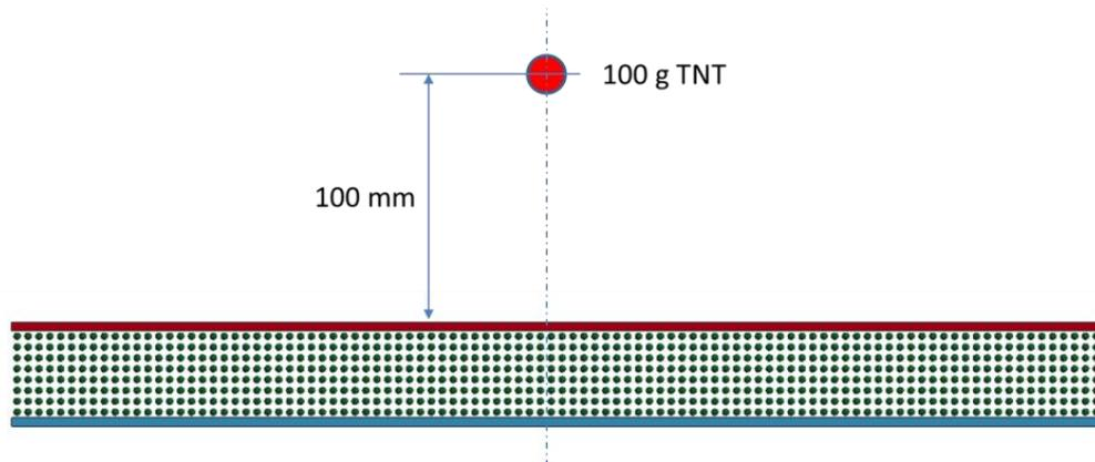
Figure 11: Blast load experiment setup
