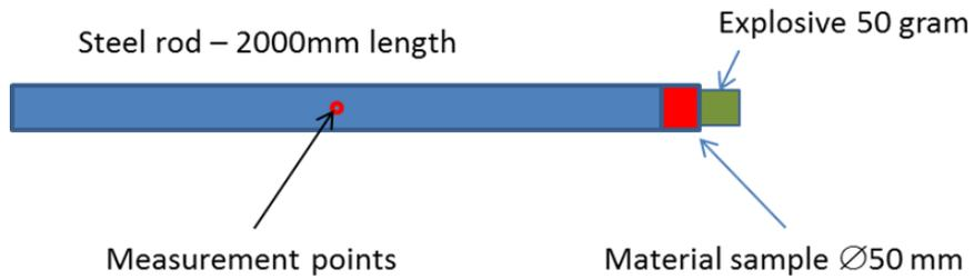
Figure 8: Scheme of explosive load experimental setup
