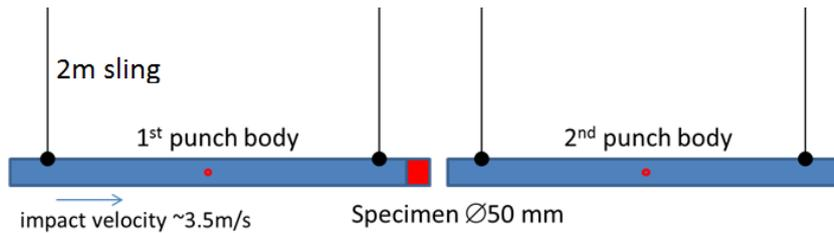
Figure 3: Scheme of “Newton Cradle“ experimental setup
