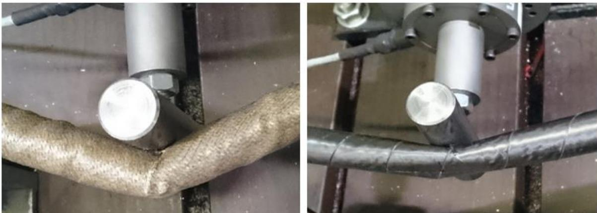
**Fig. 2** Shape of the deformed samples: a) flax fiber tube, b) carbon fiber tube
