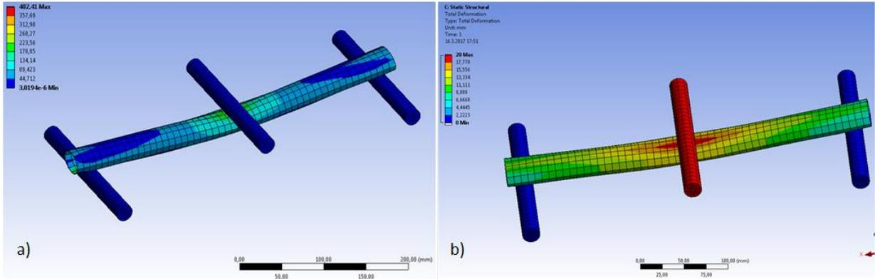
**Fig. 5** Results of the carried simulation for the stacked layer a) The Equivalent stress, b) Directional displacement
