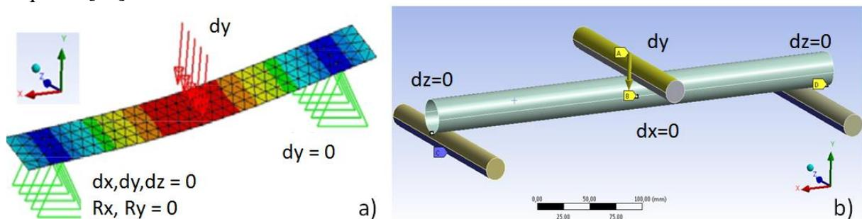
**Fig. 4** Model of bending test: a) Simplified according to [8], b) Fully defined contact model
