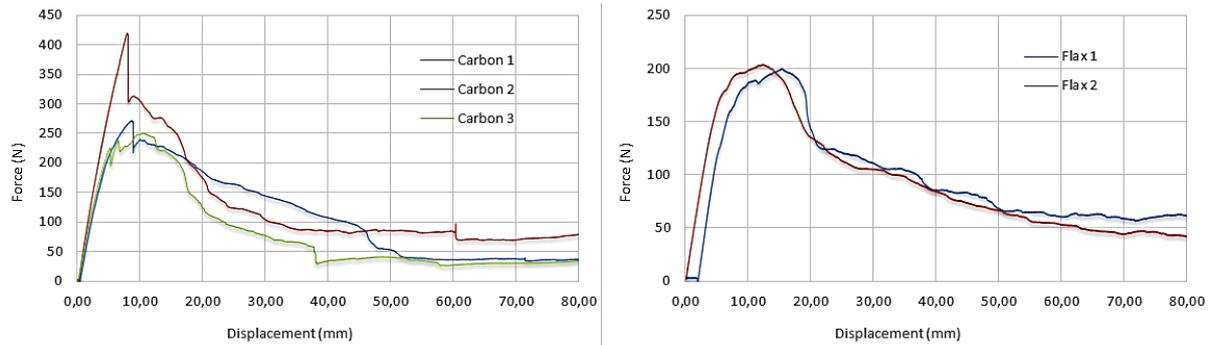
**Fig. 3** Experiment, Force – Displacement relation for the tested rods a) Carbon b) Flax
