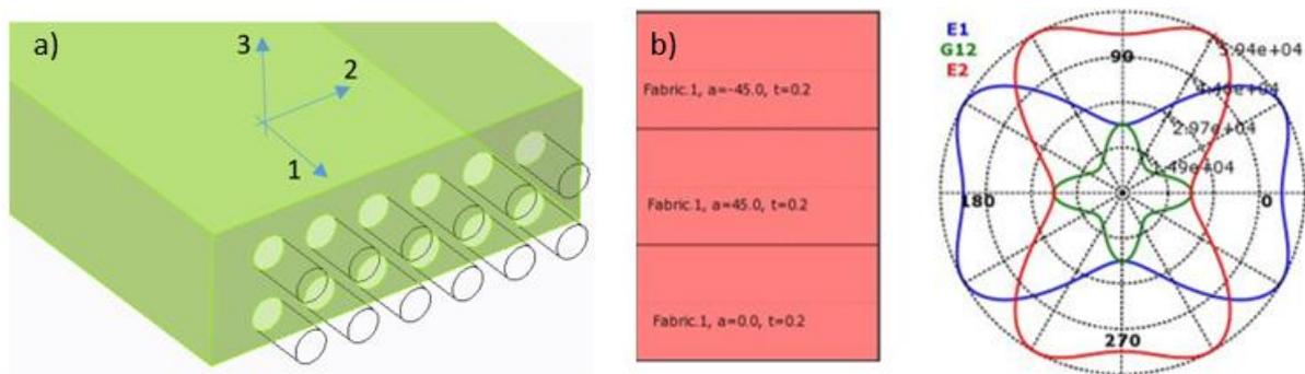
**Fig. 1** UD composite: a) Convention of the global coordinate axis b) Polar properties of the created carbon stackup (45, 0,-45)
