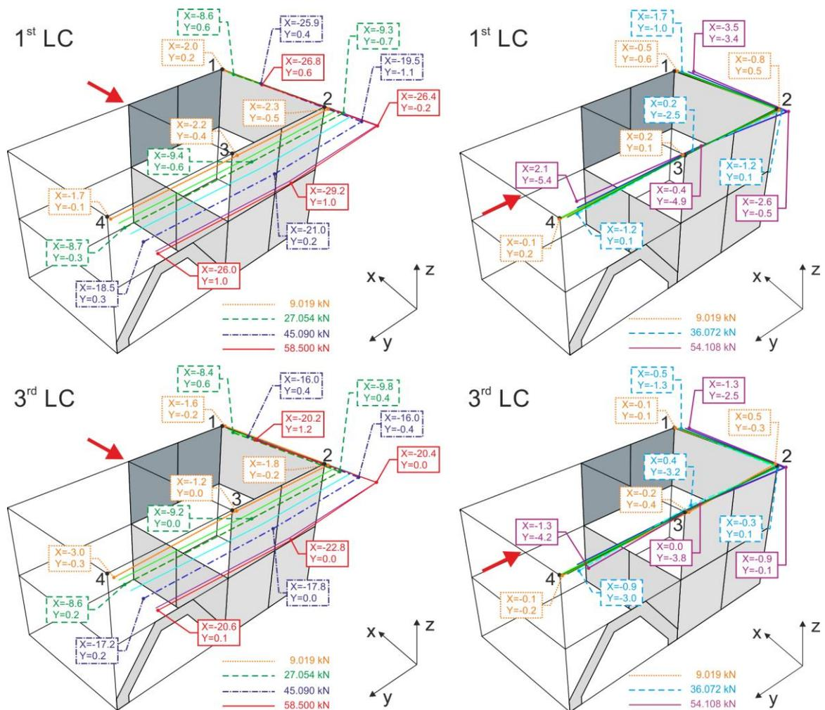
Fig. 5 Measured deformations for individual load steps (1<sup>st</sup> and 3<sup>rd</sup> load cycle)
