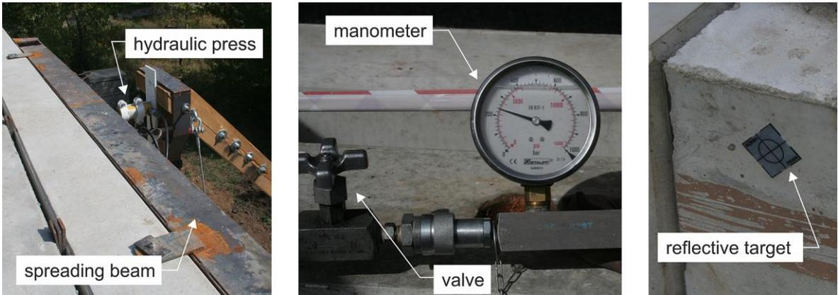
Fig. 2 Details of the test assembly
