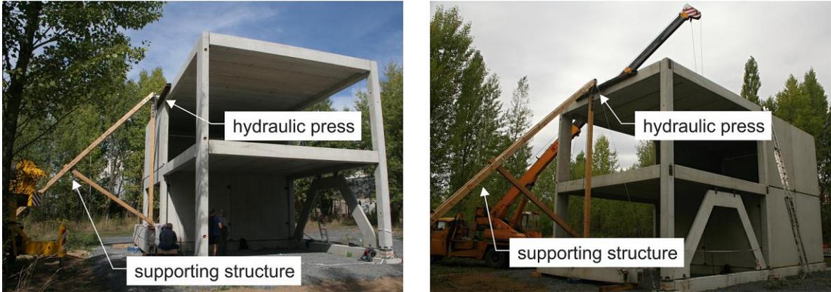
Fig. 1 Horizontal static loading in transverse (left) and longitudinal direction (right)
