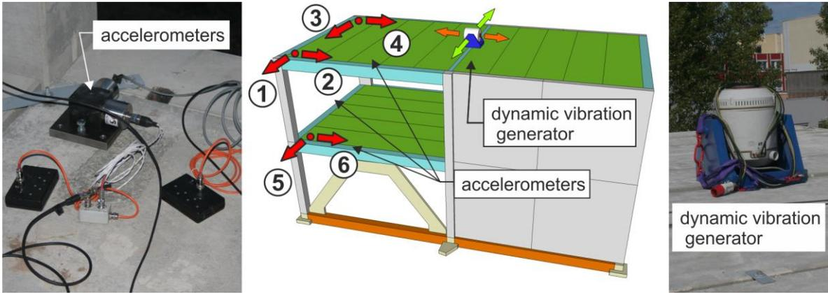
Fig. 3 Placement of accelerometers and dynamic vibration generator
