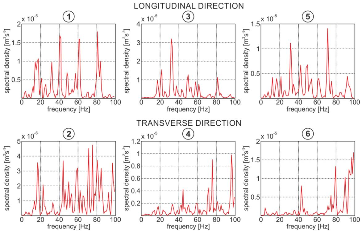
Fig. 4 Response spectrum identification of natural frequencies before the dynamic loads
