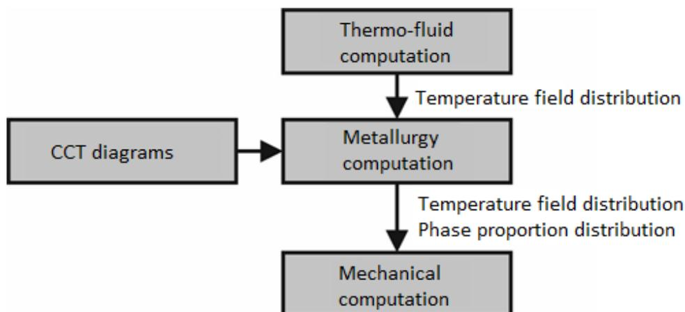
Fig.1. - Sequence scheme of friction stir welding computation
