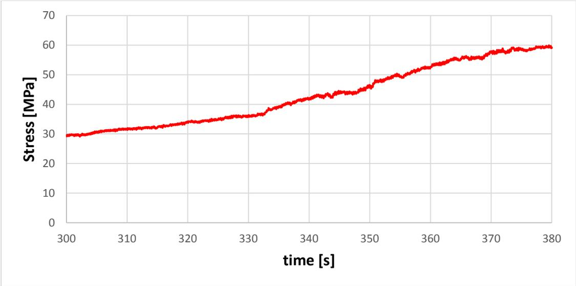
Fig. 6. – Stress state according to the Von Mises theorem obtained from measurement
