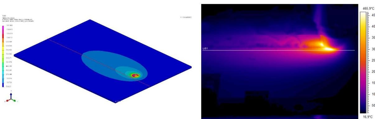
Obr. 2 – Comparison of temperature distribution of a simulation and measurement in time  $t = 374$  s
