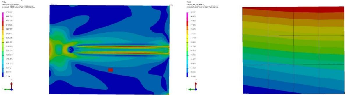
Fig.5. - Von Mises stress distribution in time  $t = 374$  s, right – detail of measured locality  $\sigma_{min} = 53,55$  MPa,  $\sigma_{max} = 82,91$  MPa
