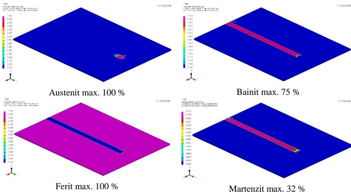
Fig.4. - Phase proportion distribution in time  $t = 374$  s
