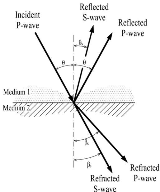
Figure 1. Reflection and refraction of P-wave [5].
