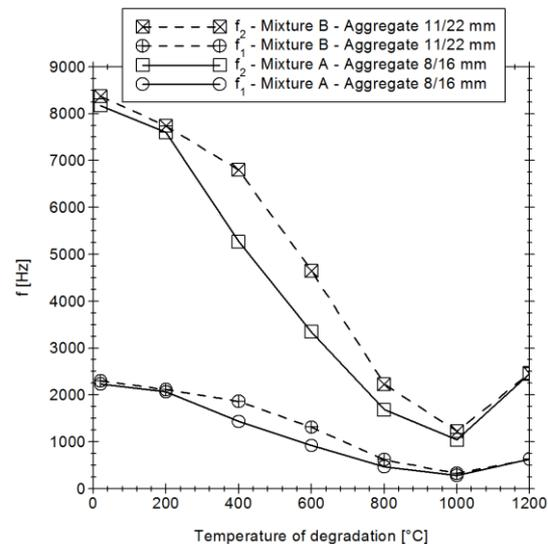
Figure 11. Dominant frequency for each mixture in transverse way.
