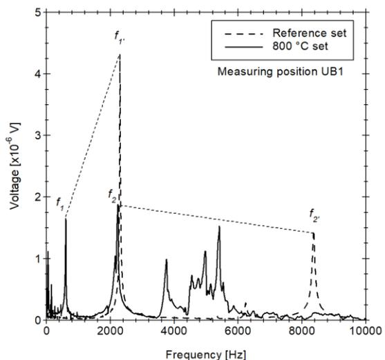
Figure 6. Shift of dominant frequency in transverse way of measurement.
