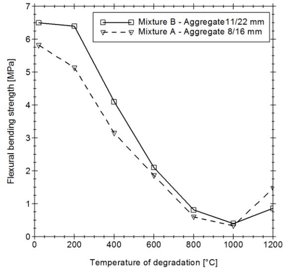
Figure 9. Flexural bending strength test.
