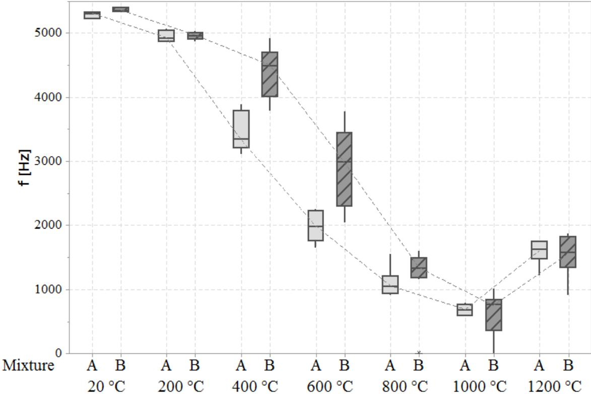
Figure 7. Measured dominant frequencies for mixture A and B in measurement position UB0.
