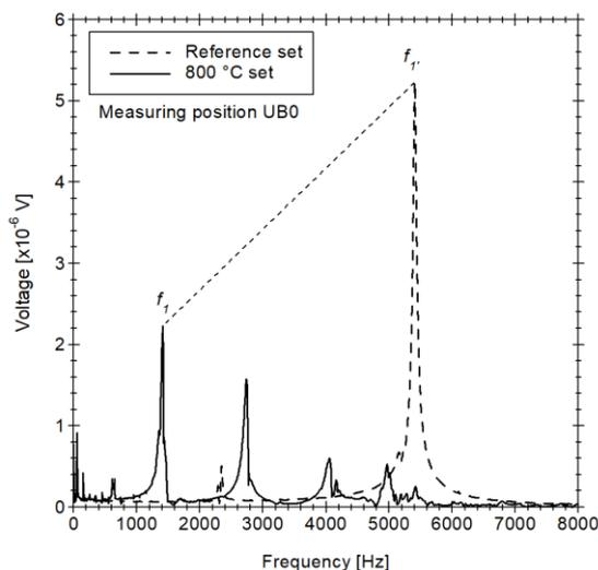
Figure 5. Shift of dominant frequency in longitudinal way of measurement.
