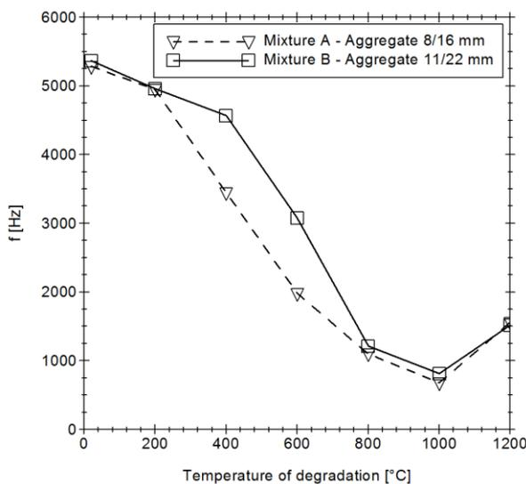
Figure 10. Dominant frequency for each mixture in longitudinal way.
