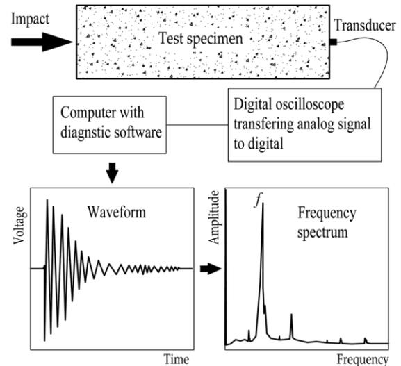
Figure 4. Diagram of measuring process.
