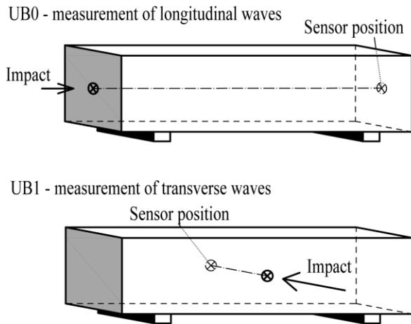
Figure 3. Impact-echo measuring positions.
