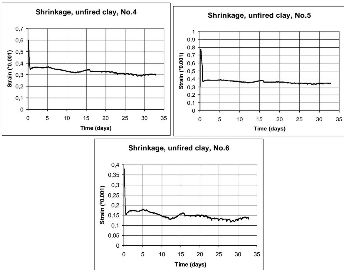
Fig.4 The curves of the shrinkage on the specimens 4-6 prepared from described clay.
