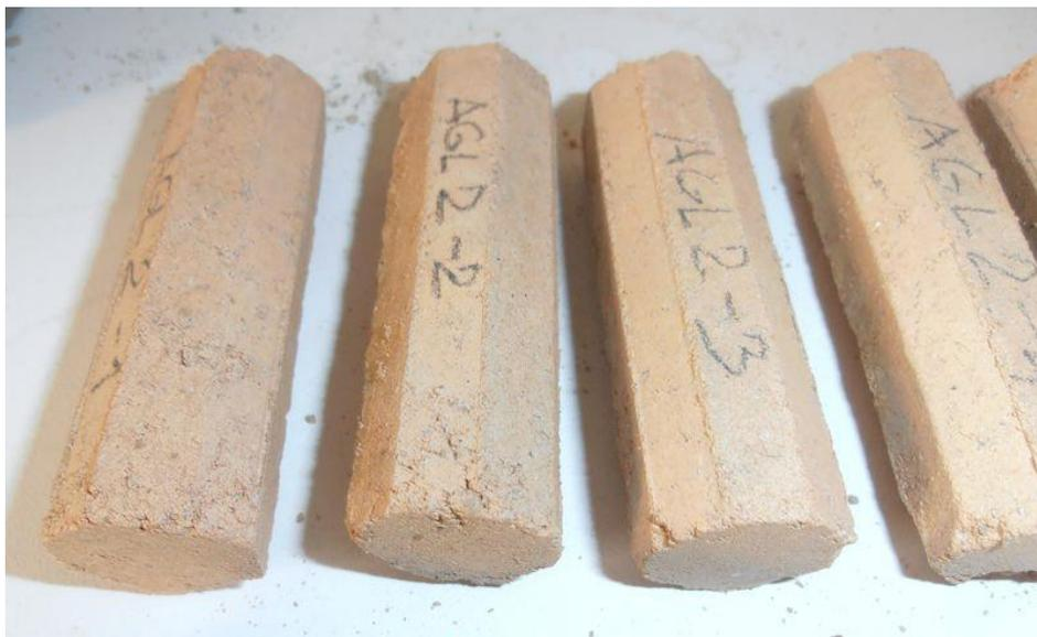
Fig.1 The specimens used for measurement of creep and shrinkage, prepared from illitic clay.
