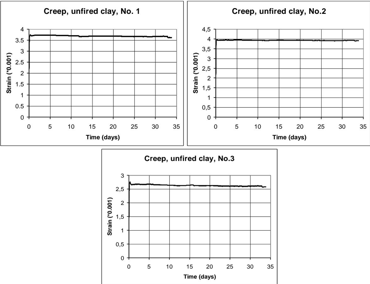
Fig.3 The curves of the creep measured on the specimens 1-3 prepared from described clay.
