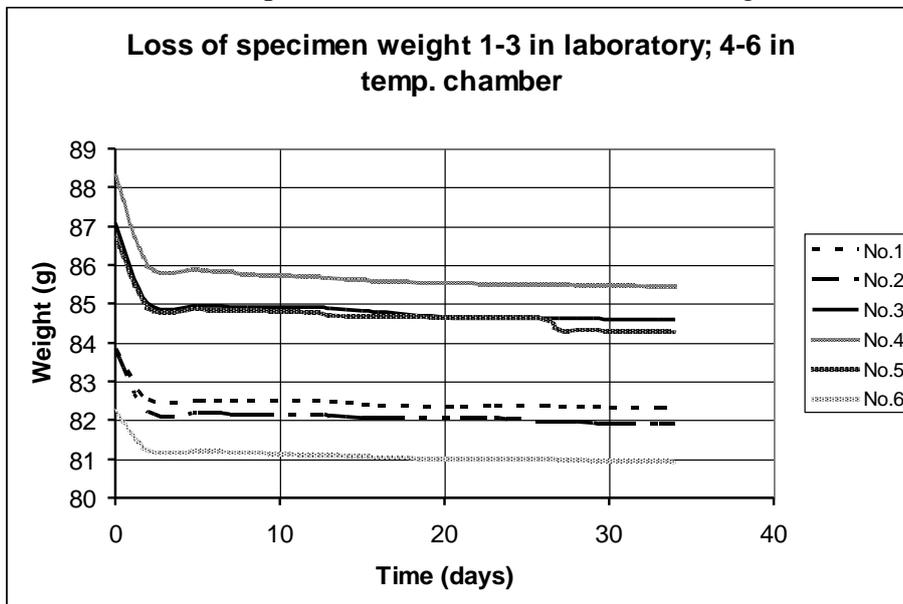
Fig.6 The change of the weight of specimens during the test.
