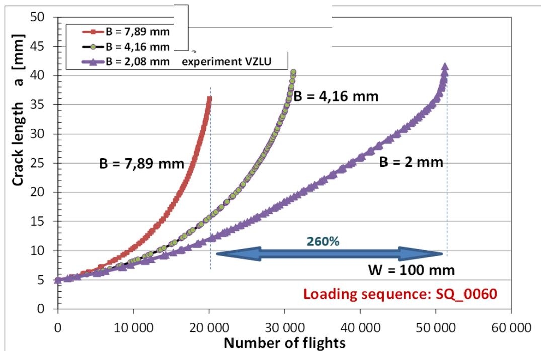
Fig. 5 7475 T7351 crack propagation data comparisons under variable amplitude loading conditions  $\sigma_{\max} = 89$  MPa – effect of thickness
