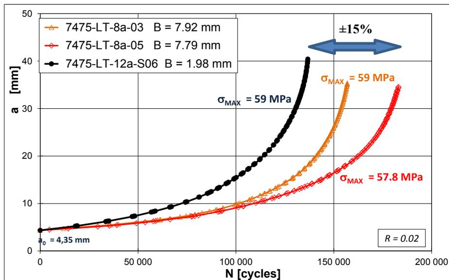
Fig. 4 7475 T7351 crack propagation data under constant amplitude loading – effect of thickness
