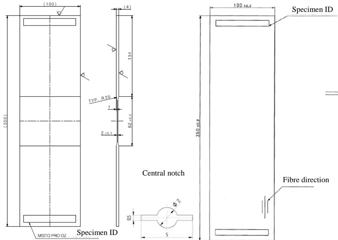
Fig. 1 M(T) specimen geometry (left - thickness of 2 mm, right - thicknesses of 4 and 8 mm)
