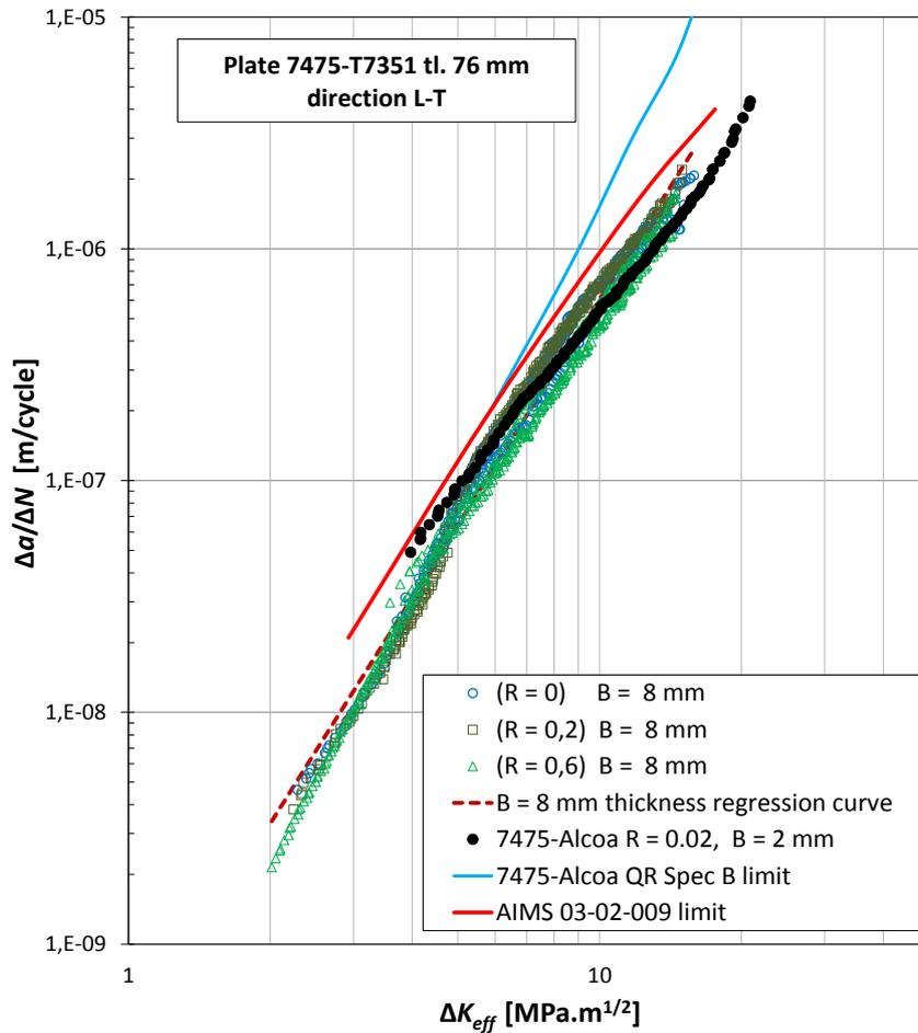
Fig. 3 7475 T7351 crack rate vs. effective stress intensity factor data – effect of thickness
