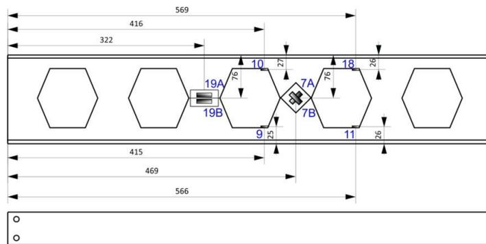
Fig. 11 Position of the resistance strain gauges on the CGH
