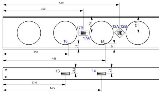
Fig. 10 Position of the resistance strain gauges on the CGC
