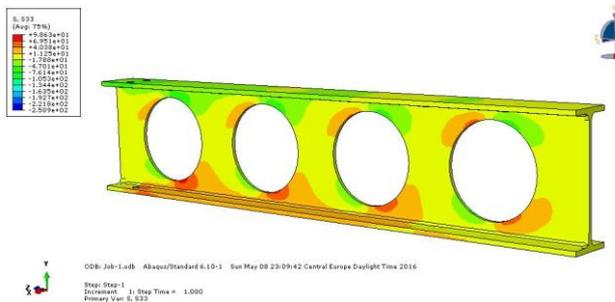
Fig. 18 Field of normal stresses  $\sigma_z$  in the CGC
