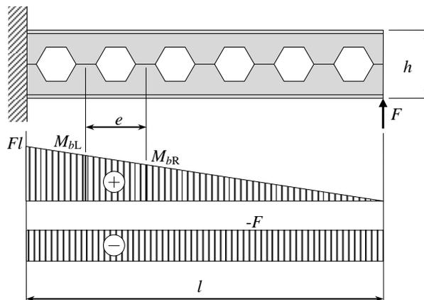
Fig. 6 Loading force  $F$ , bending moment  $M_b$  and shear force along the castellated beam
