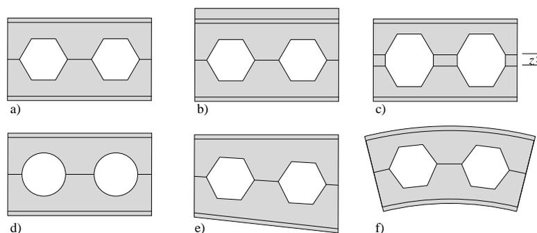
Fig. 4 Basic and special shapes of the castellated girders
