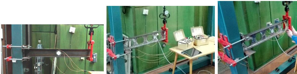
Fig. 8 Experimental model of the IPE 100, CGC, CGH and respective experimental chain and loading unit
