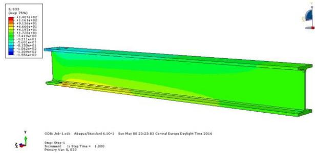
Fig. 17 Field of normal stresses  $\sigma_z$  in the IPE 100
