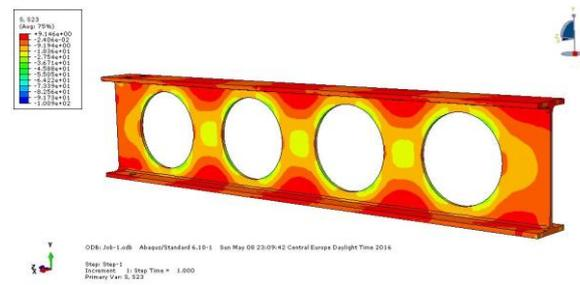
Fig. 15 Field of shear stresses  $\tau_{zy}$  in the CGC
