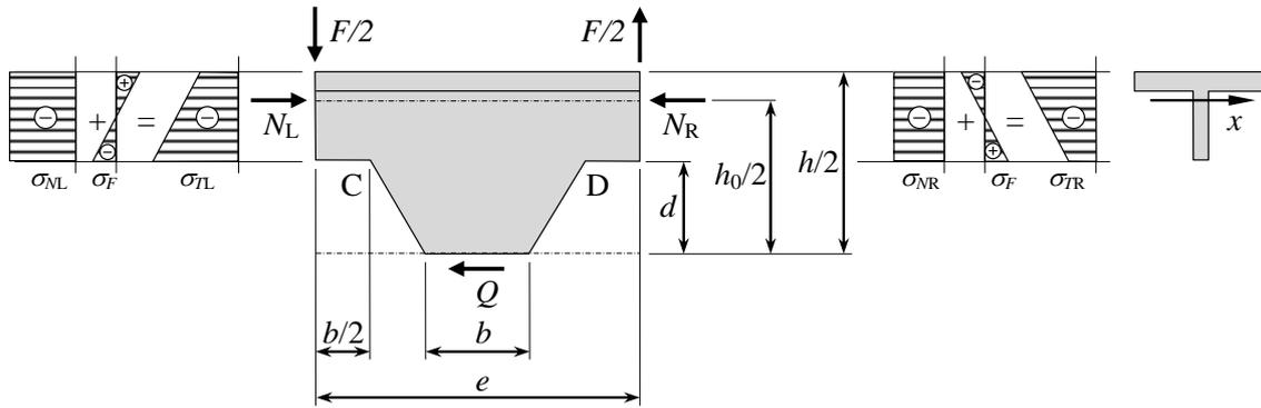
Fig. 7 Preparing of the castellated beam CGH to analytical solution
