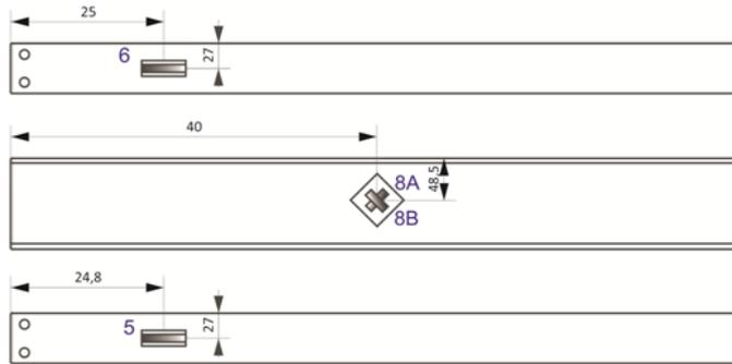
Fig. 9 Position of the resistance strain gauges on the IPE 100
