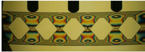
Fig. 13 Field of isochromatics in the CGH [5]
