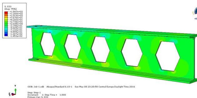
Fig. 19 Field of normal stresses  $\sigma_z$  in the CGH
