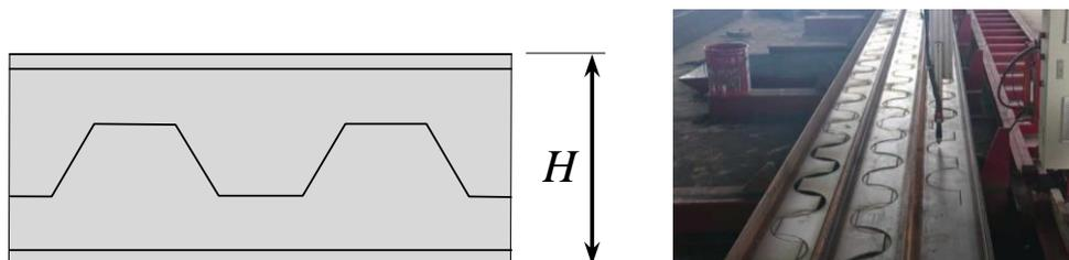
Fig. 1 Creating castellated girders using cutting and welding [1]
