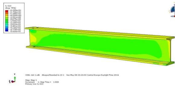
Fig. 14 Field of shear stresses  $\tau_{zy}$  in the IPE 100
