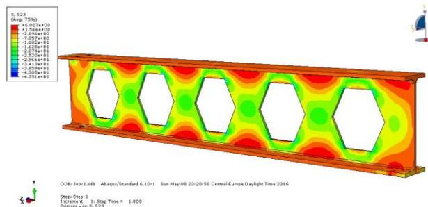
Fig. 16 Field of shear stresses  $\tau_{zy}$  in the CGH
