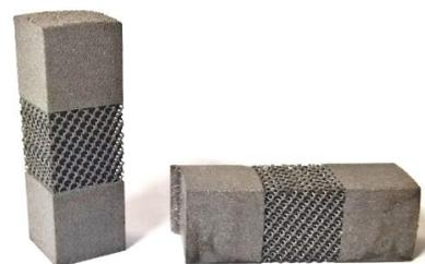
b) tensile test specimen
