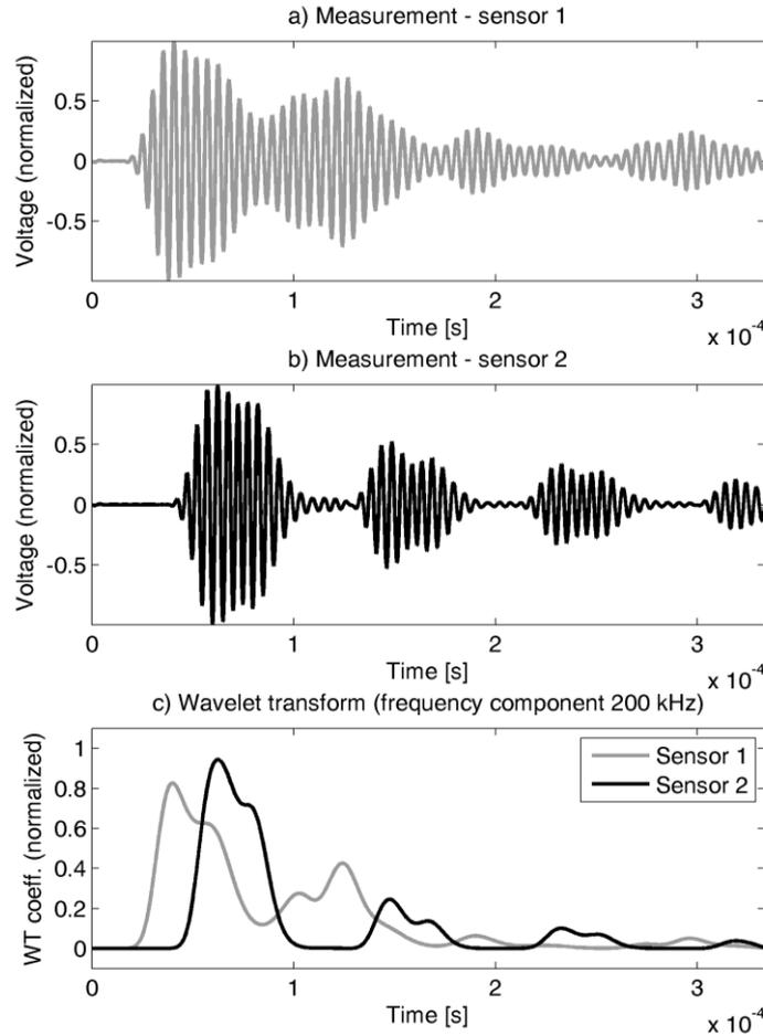
Fig. 3 Time records from a pair of sensors (a, b) and time history of frequency component 200 kHz (c).
