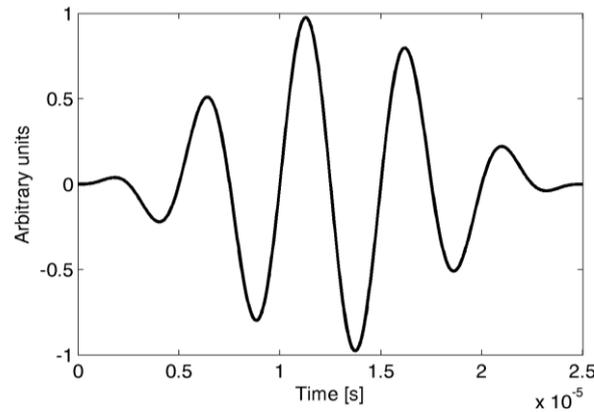
Fig. 2 Five-cycle sine burst with frequency 200 kHz
