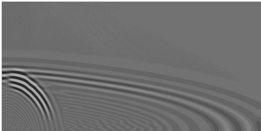
Fig. 5 Out-of-plane displacement of the plate in time  $t = 180$  ms from numerical analysis.
