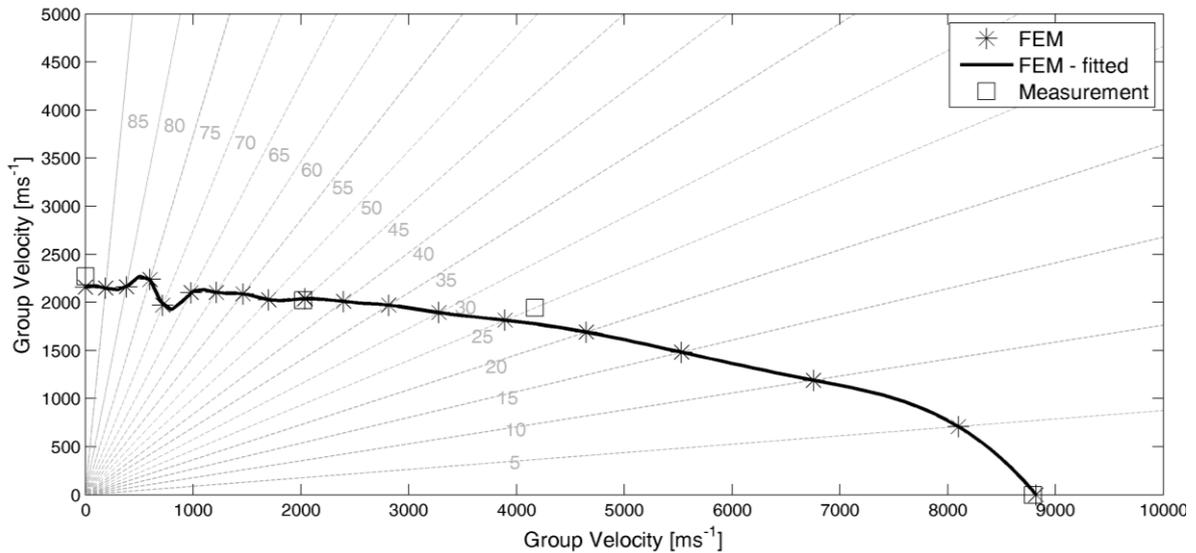
Fig. 4 Angular dependency of group velocity of  $S_0$  mode (frequency 200 kHz).
