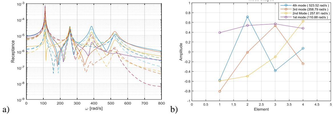
Fig. 2 a) FRFs of the system, b) Mode shapes of vibration.
