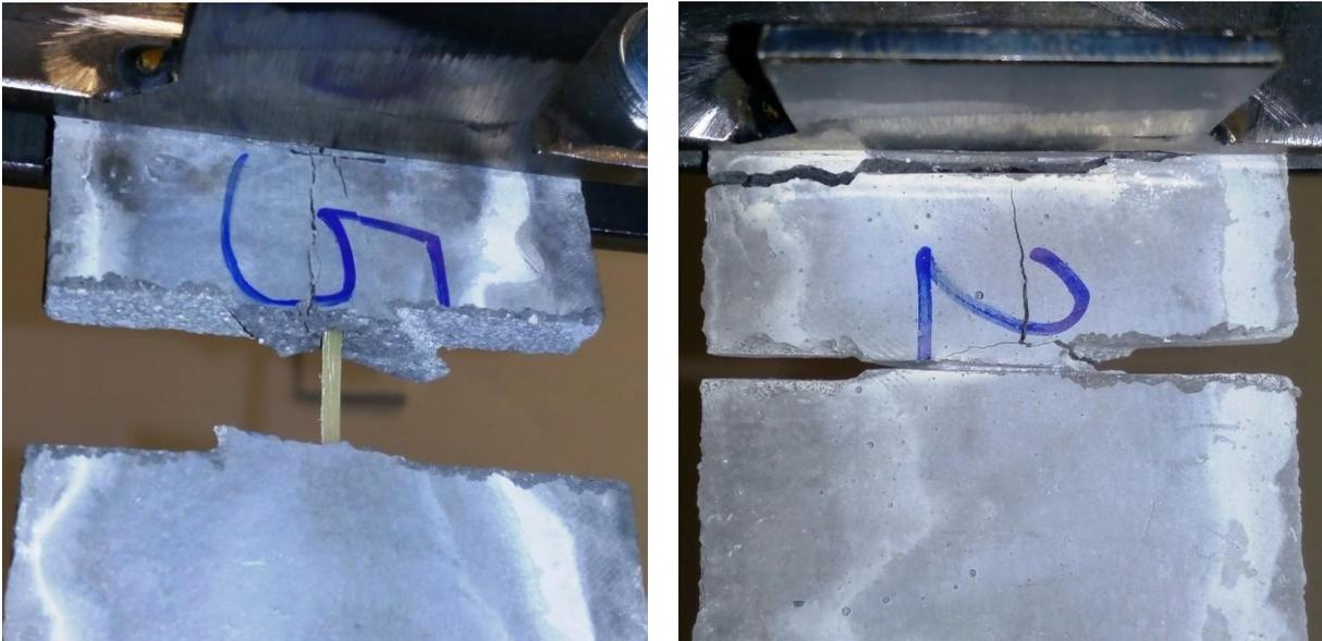
Fig. 3: The difference between specimens with and without surface treatments, pictures were made immediately after the test was interrupted due to the sample breaking.
