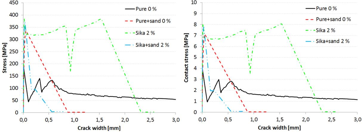
Fig. 2: Tensile stress in composite reinforcement and contact stress between composite reinforcement and cement matrix depending on the crack width development.
