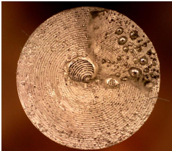
Fig.6 Bubbles inside solder area
