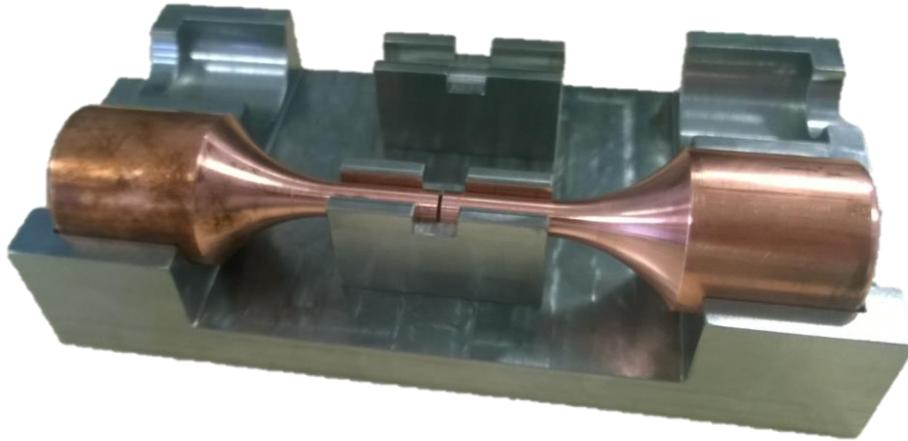
Fig.3 Soldering tool with copper parts of final specimen
