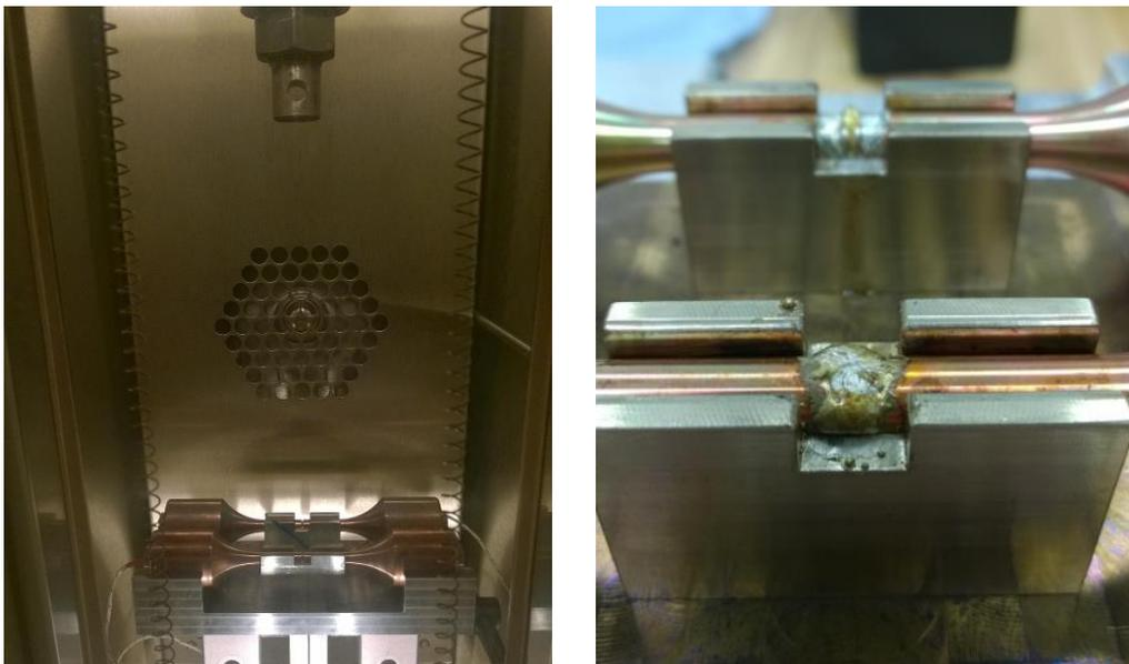
Fig.4 Soldering at temperature chamber on the left and cooling after soldering on the right
