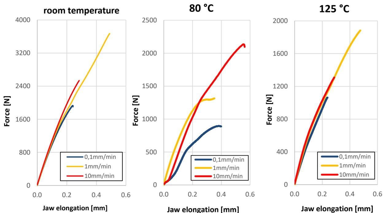
Fig.9 tensile tests records
