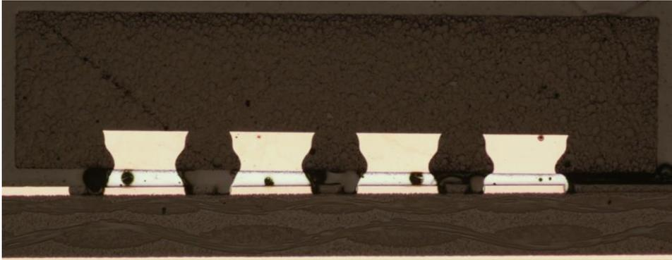
Fig.7 Bubbles inside solder joint
