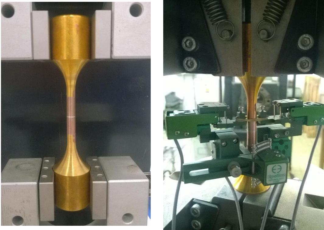
Fig.8 Fixture of specimen during tension test (left) and torsion test (right)
