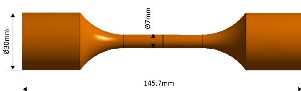
Fig.2 Solder paste specimen
