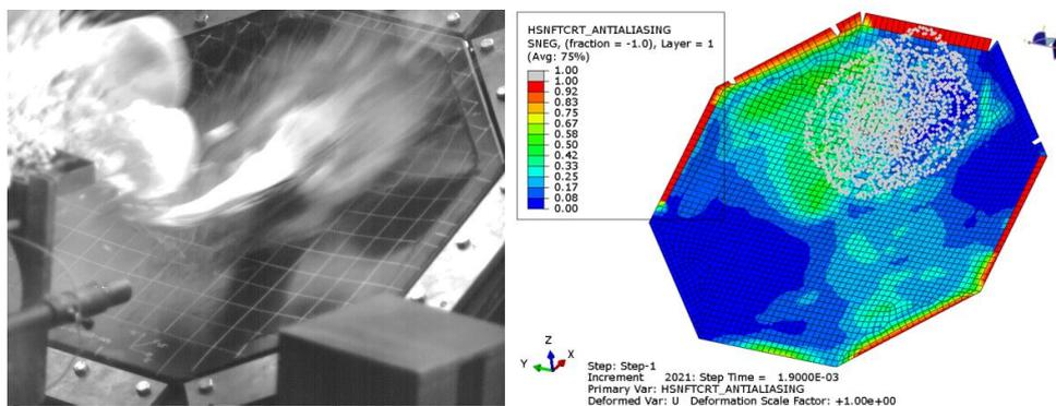
Fig.2 Bird strike test on flat test composite panel (left) and numerical simulation (right) [4]
