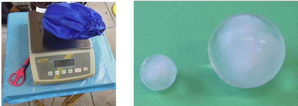
Fig.5 Weighting of bird in textile bag (left) for bird strike test and ice balls (25 mm and 50 mm) for hail strike tests
