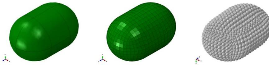
Fig. 10 Geometric model (left), FE mesh (centre), and SPH elements (right), of the idealised bird
