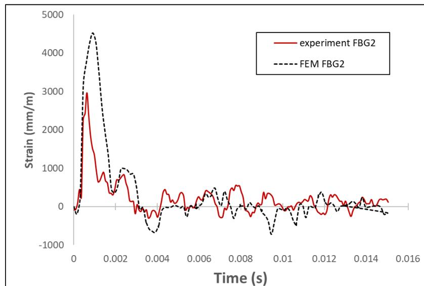
Fig.21 comparison between strain measurement on FBG sensors and numerical simulation for sensors FBG2 (see figure 9)
