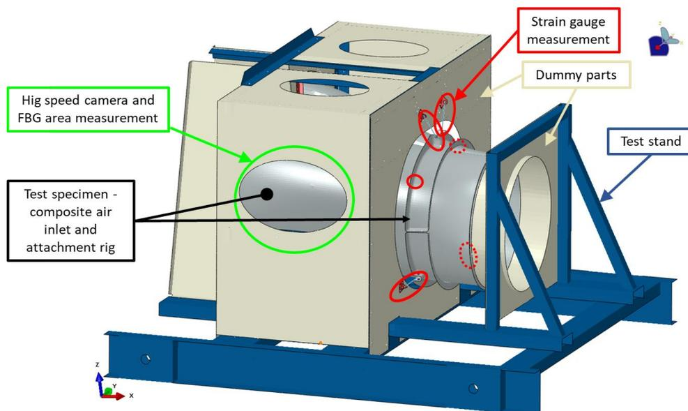
Fig.7 Shema of impact test assembly and measurement
