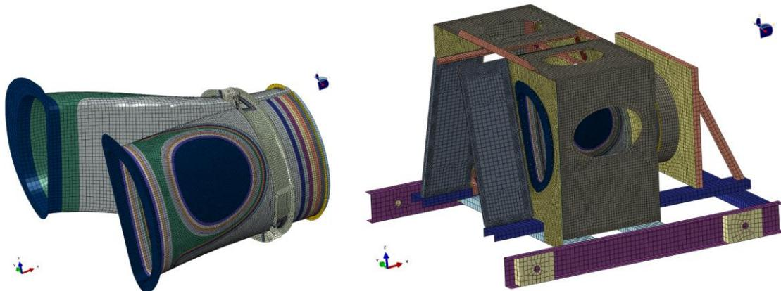
Fig.11 FE model of composite inlet (left) and FE model of test assembly (right)
