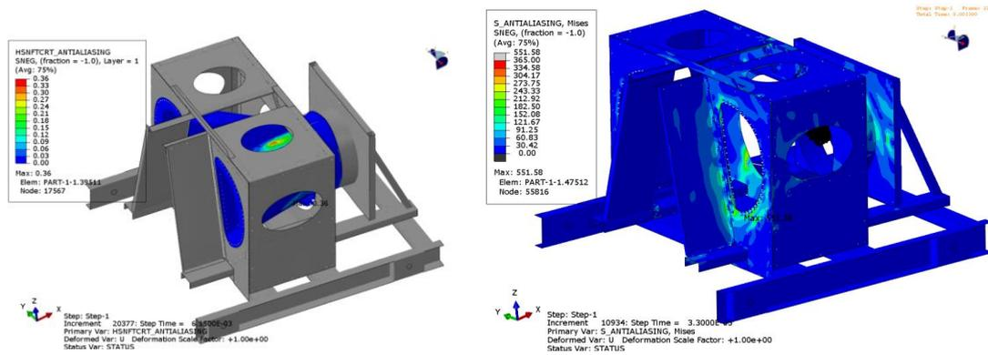
Fig. 12 FE analysis of composite parts (left) and test rig with dummy parts (right)
