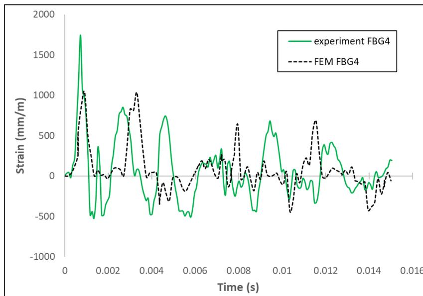
Fig.23 comparison between strain measurement on FBG sensors and numerical simulation for sensors FBG4 (see figure 9)
