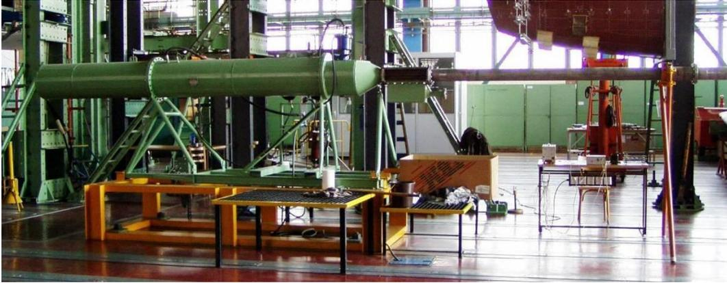
Fig. 4 VZLU air gun used for high speed impact tests
