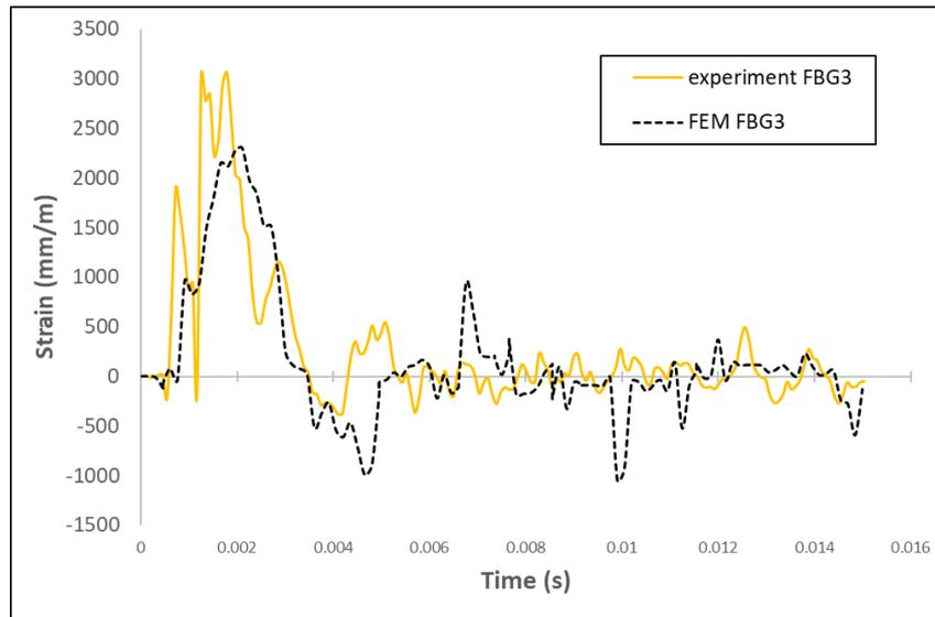
Fig.22 comparison between strain measurement on FBG sensors and numerical simulation for sensors FBG3 (see figure 9)
