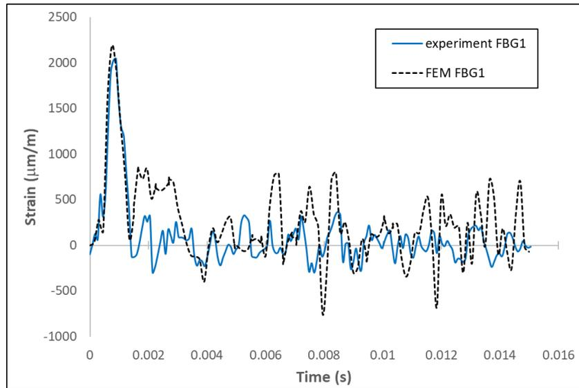
Fig.20 comparison between strain measurement on FBG sensors and numerical simulation for sensors FBG1 (see figure 9)
