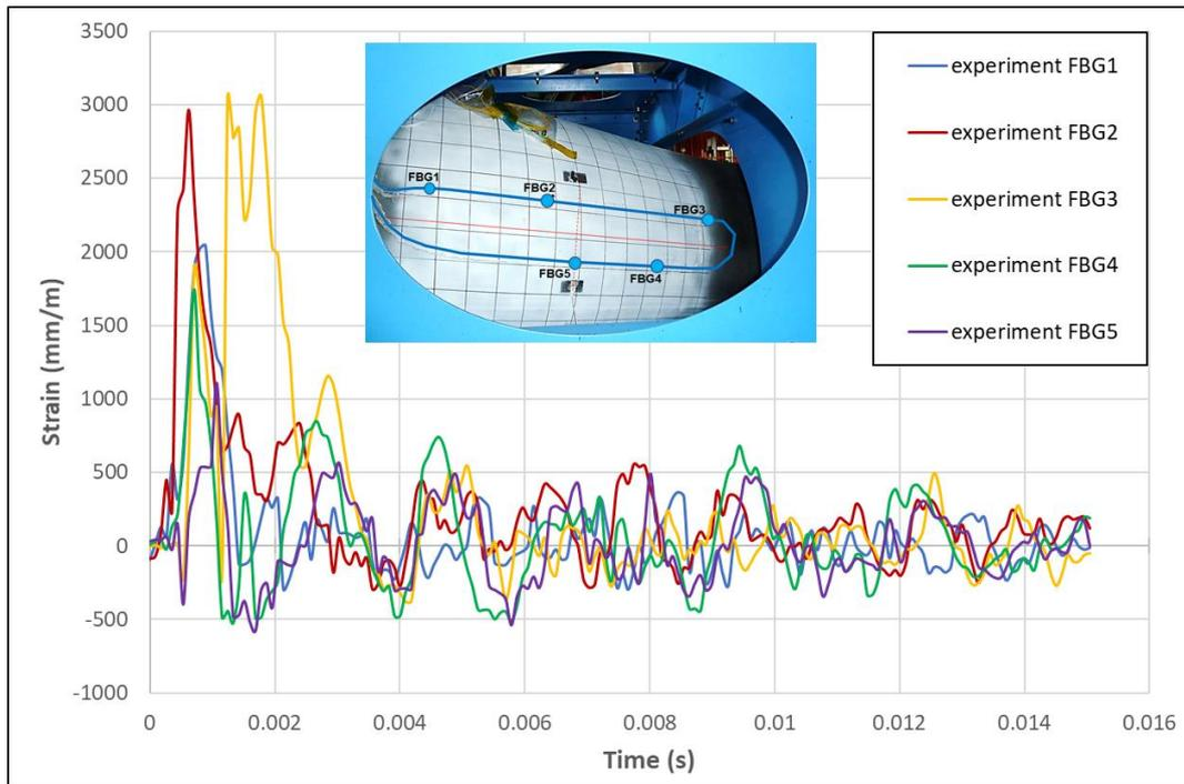
Fig.14 Strain measurement by FBG sensors during impact (CTU) [10]
