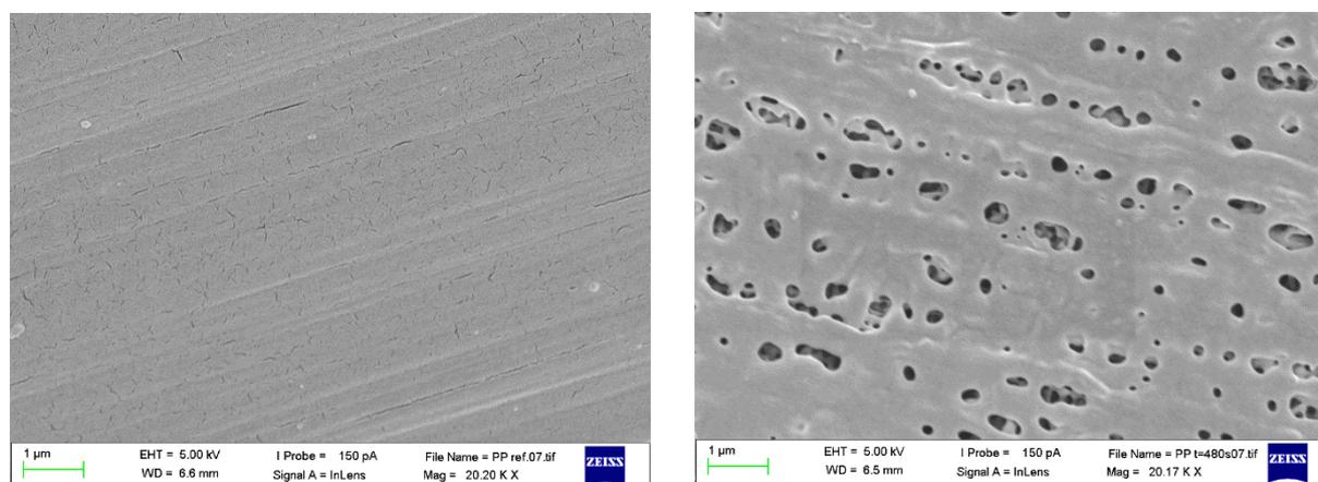
Fig.1 Comparison of fibre surface, reference – left, plasma modified surface at 480 seconds - right
