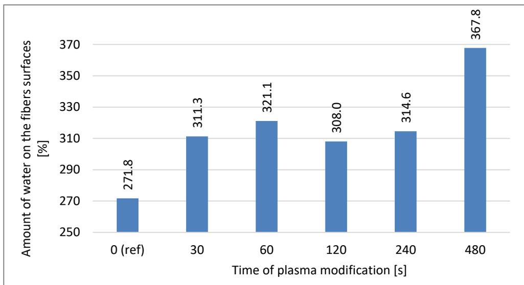
Fig.2 The weight of water between the fibers
