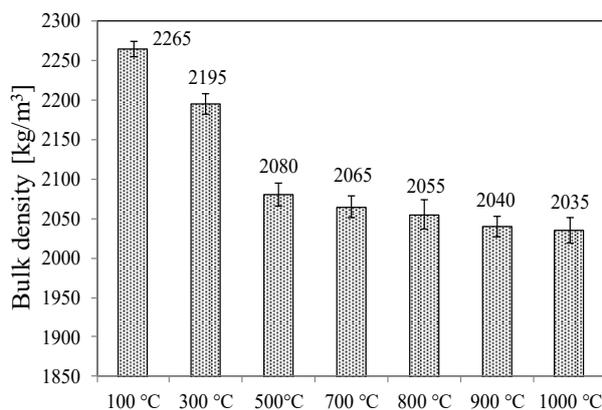
Fig.1 Evaluation of bulk density
