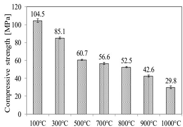
Fig.2 Evaluation of compressive strength
