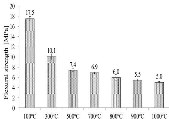
Fig.3 Evaluation of flexural strength
