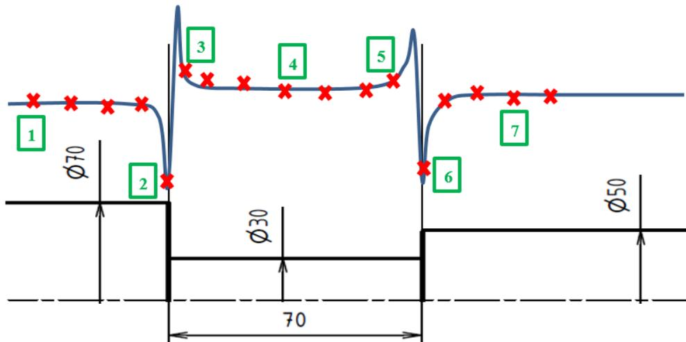
Fig. 7 Results (illustrative course of stress: x – experimental data; - - FEM)
