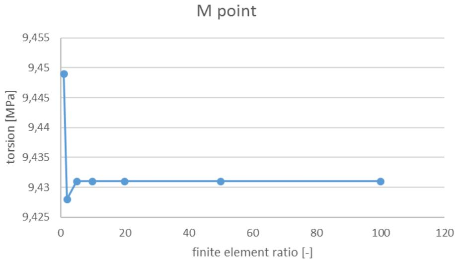
Fig. 4 Cylindrical section of 30 mm in diameter: stress vs. the element size (finite element ratio = size of the biggest element / actual size of the local element)
