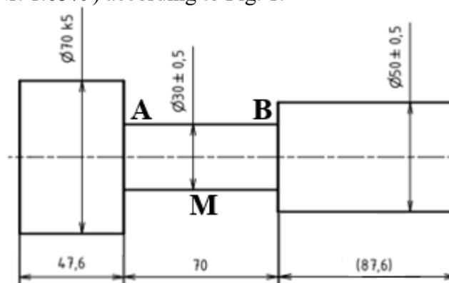
Fig. 1 Drawing of the test shaft (cut-out from the drawing)
