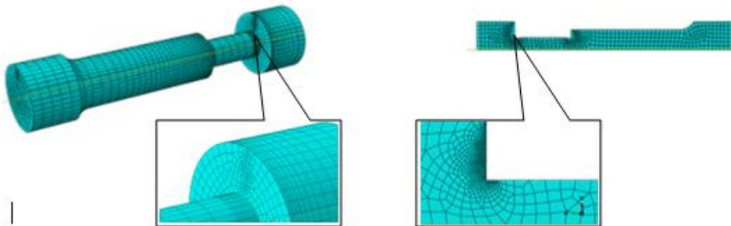
Fig. 3 3D (left) and 2D (right) model of the shaft
