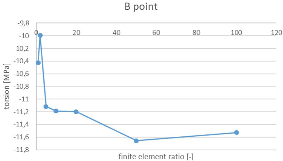
Fig. 6 Notch B, shaft shoulder 30 per 50 mm: stress vs. the element size (finite element ratio = size of the biggest element / actual size of the local element)
