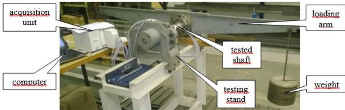
Fig. 2 Measurement work station setup
