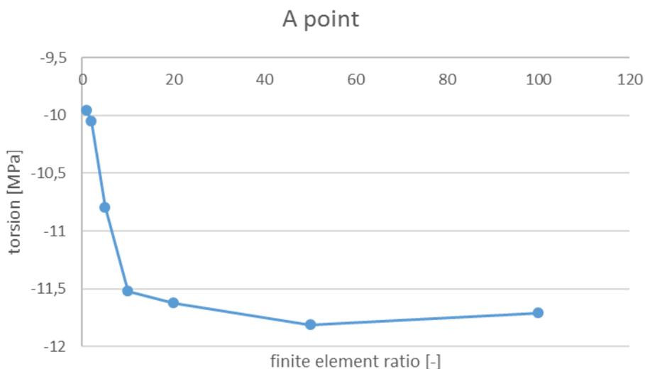
Fig. 5 Notch A, shaft shoulder 70 per 30 mm: stress vs. the element size (finite element ratio = size of the biggest element / actual size of the local element)
