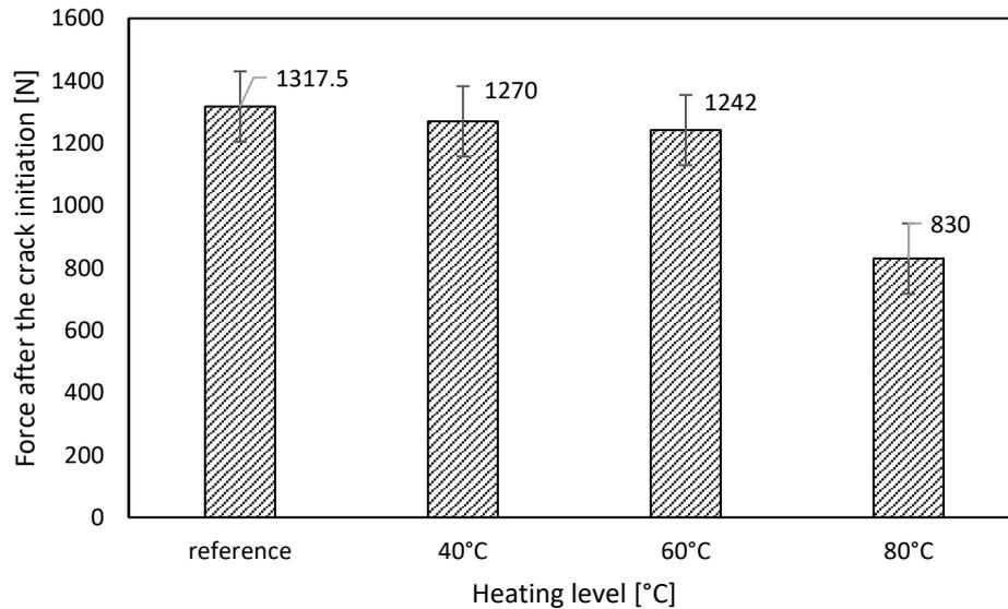
Fig. 1 Force in textile reinforcement after the crack initiation
