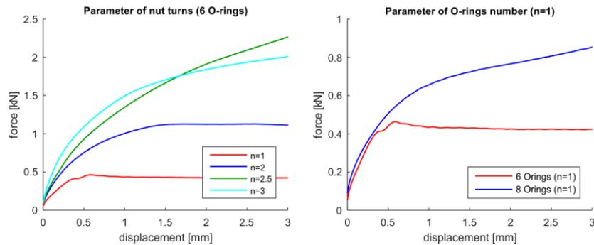
Fig. 7 Measured data for different locking parameter and number of O-rings
