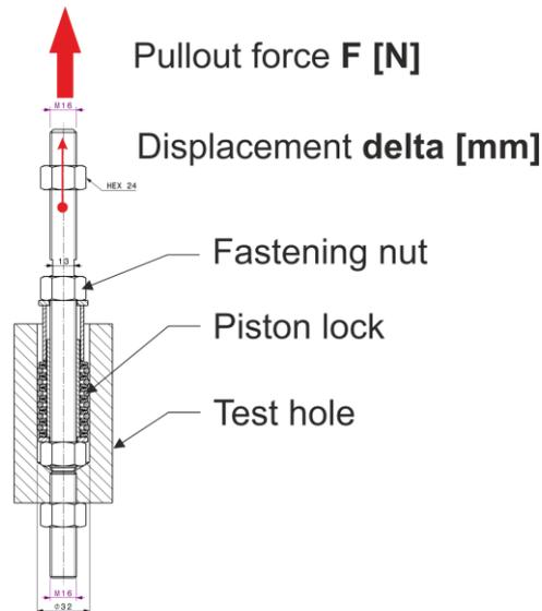
Fig. 2 Scheme of tested specimen
