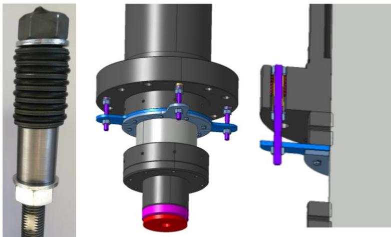
Fig. 1 Tested specimen (piston lock)
