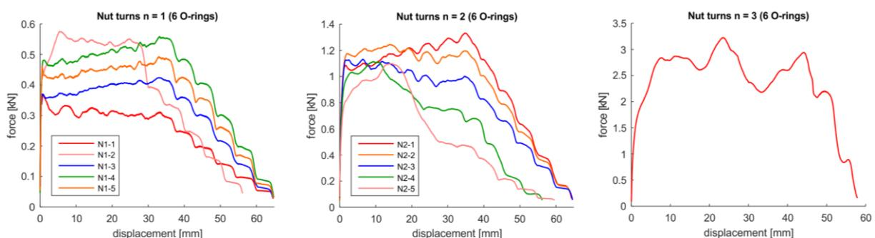
Fig. 6 Measured data for different locking parameter of nut turns
