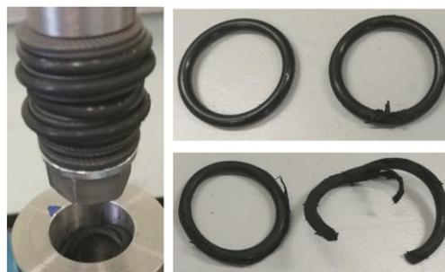
Fig. 5 Crushing and loss of O-rings
