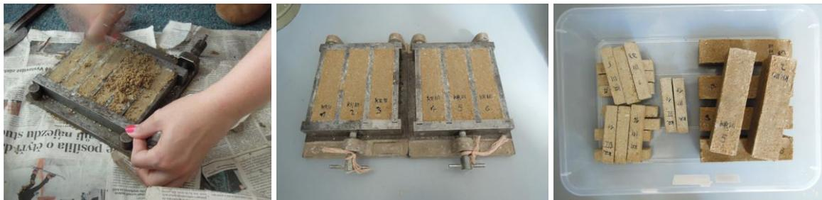
Fig.3 The produce of specimens in laboratory.
