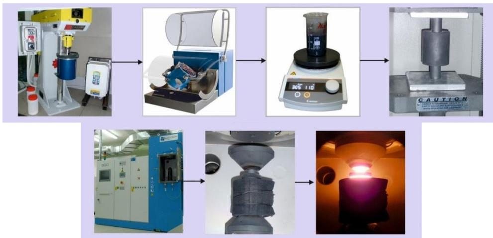
Fig. 39 Scheme of creation technology of cutting ceramic sample: refinement powders (wet grinding) – evaporation – pressing – sintering
