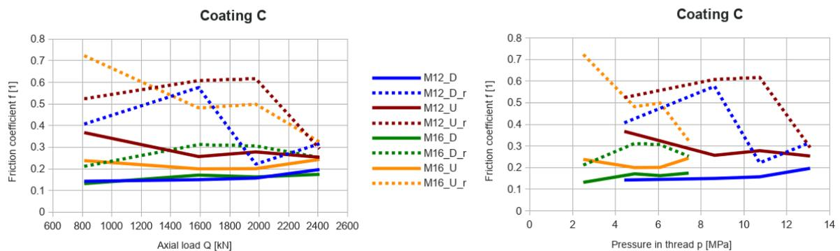
Fig 5 Friction dependence on axial load and pressure in the thread for coating C
