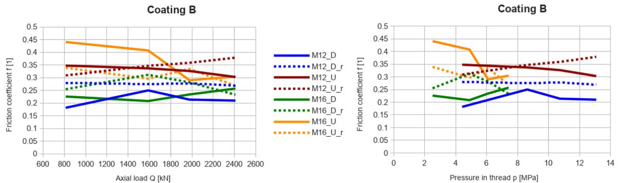
Fig 4 Friction dependence on axial load and pressure in the thread for coating B
