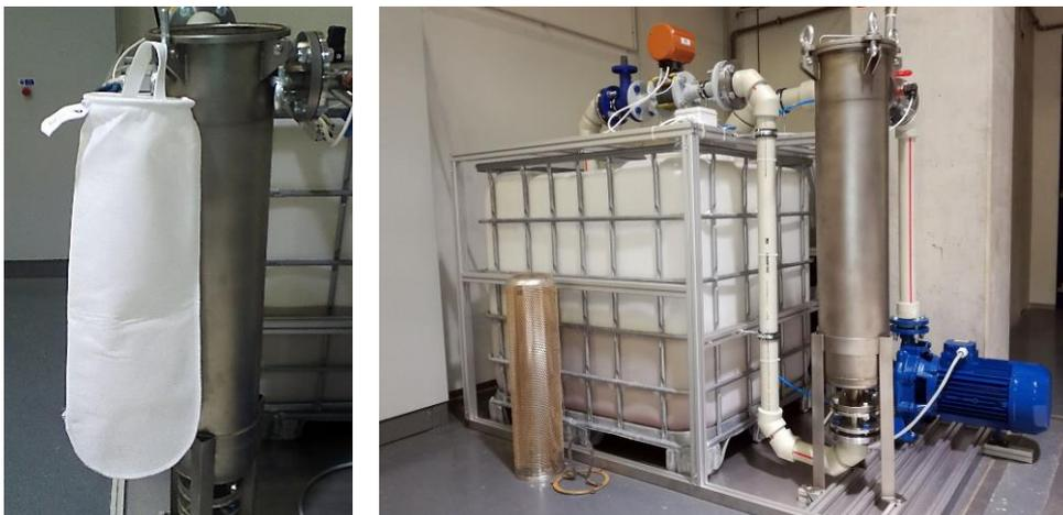
Fig. 1 and 2 Sleeve filter (left), filtration line (right)
