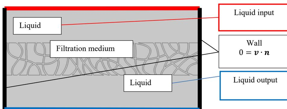
Fig. 7 Numerical model for analyzing the filter properties of the proposed media: defining of boundary conditions
