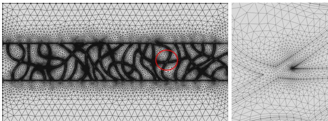
Fig. 8 and 9 Finite element mesh of the model geometry; a refinement of the mesh depends on dimension and a shape of locality
