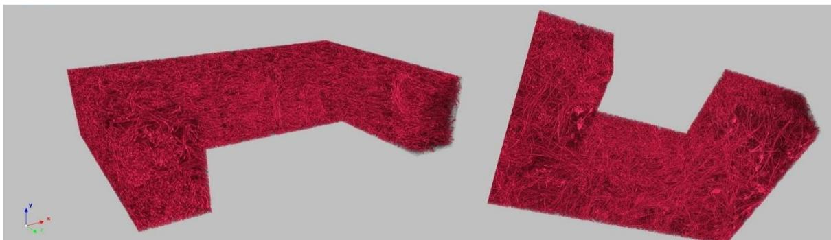
Fig. 4 The picture of fibrous filter taken by the microtomography
