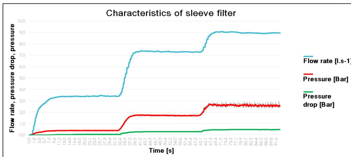
Fig. 3 Graph of filtration characteristics of the sleeve filter
