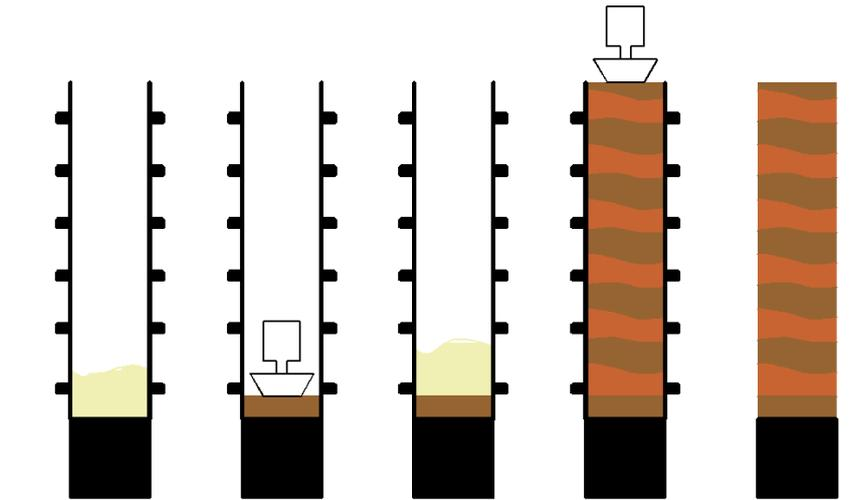
Fig. 2 Production of rammed earth
