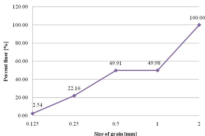
Fig. 3 Grain curve of used sand
