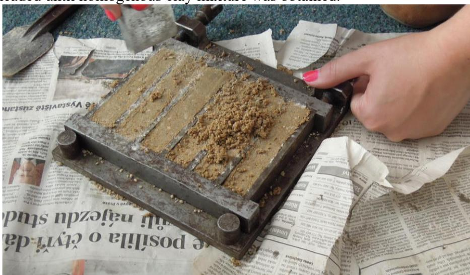
Fig. 5 Ramming of the earth mixture to the steel moulds
