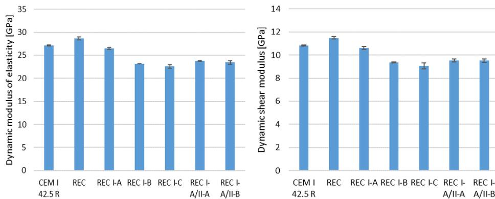
Fig.1 Comparison of dynamic modulus of elasticity and dynamic shear modulus (with standard deviations)
