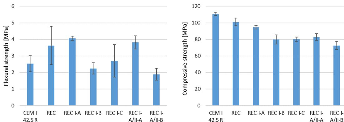
Fig.2 Comparison of flexural strength and compressive strength (with standard deviations)
