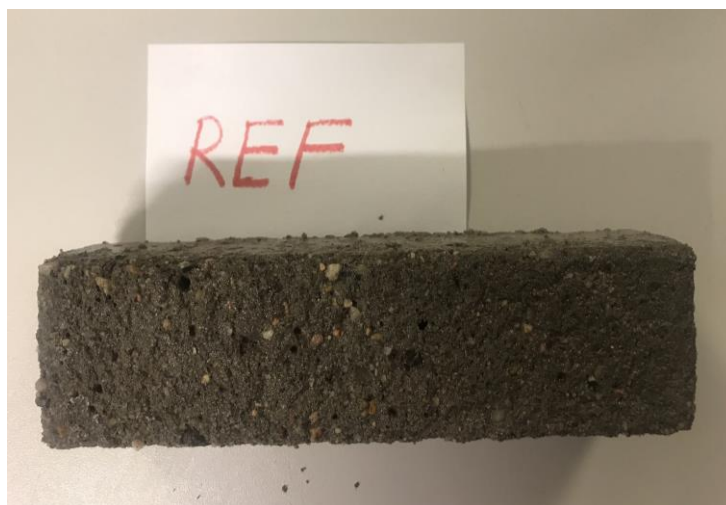
Fig. 3 Concrete surface disruption after 100 CHLR cycles – REF concrete
