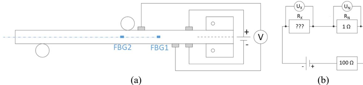
Fig. 49 Measurement procedure of the electrical resistance measurement - configuration of duty current injection and voltage change measurement on the specimen (a), schematic of the series comparison measurement method (b)
