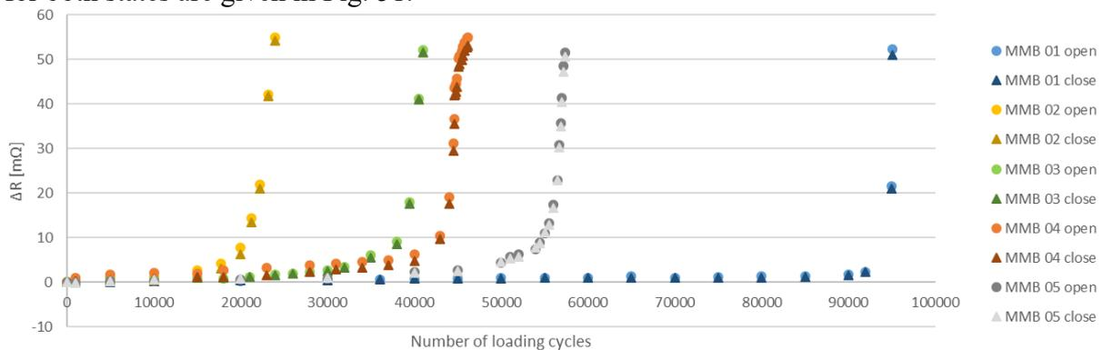
Fig. 51 Change in measured electrical resistance vs. number of cycles of all tested MMB specimens for states loaded/unloaded – opened/closed crack
