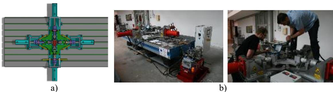
Fig. 19 Hydraulic loading equipment a) computer model, b) real model including control panel and hydraulics
