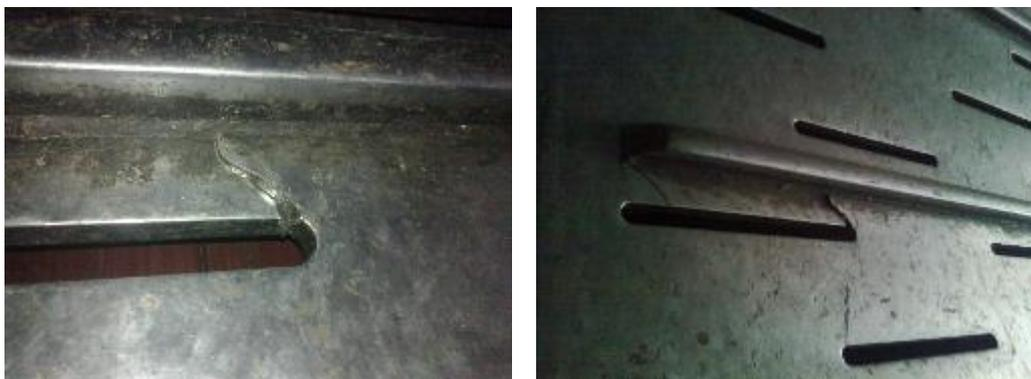
Fig. 3 Cracks on the drum beginning in the location of stress concentrator
