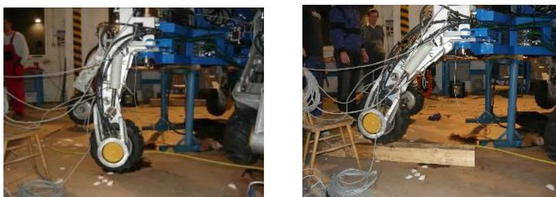
Fig. 16 Selected position of robot legs during experimental measurement.
