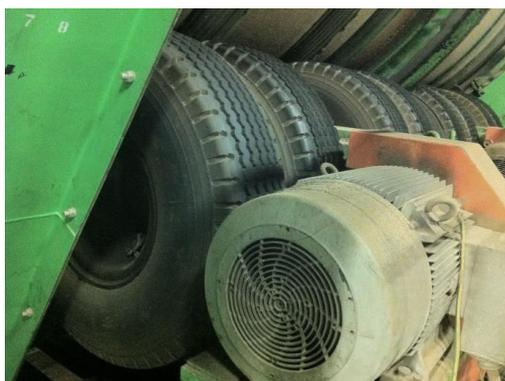
Fig. 2. Powered tyres and their connection to gearbox
