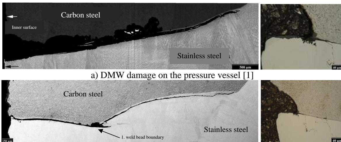
a) DMW damage on the pressure vessel [1]
