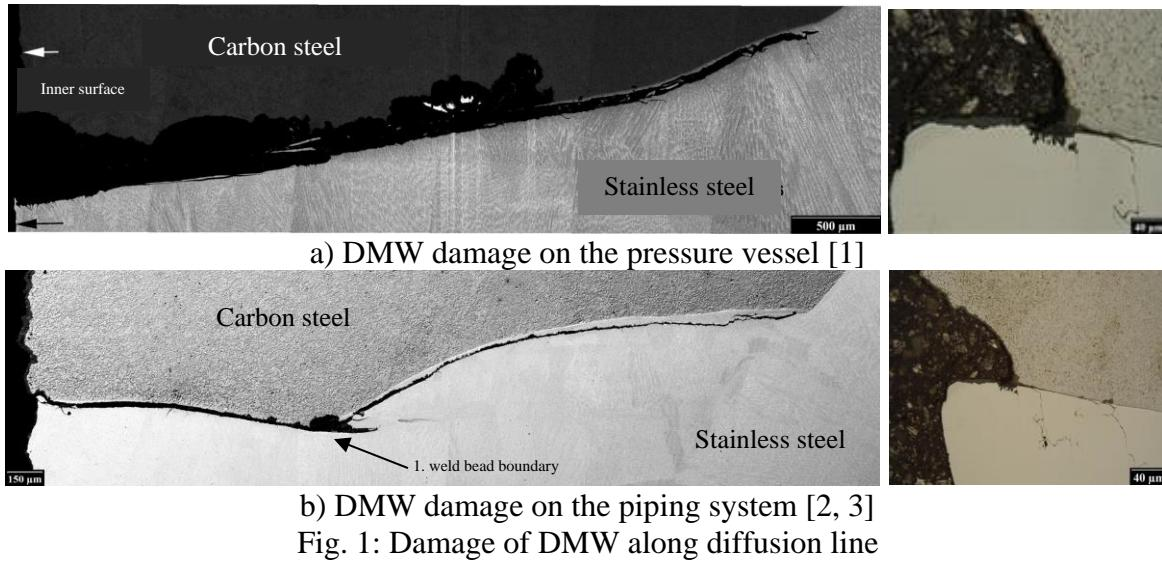
b) DMW damage on the piping system [2, 3]
