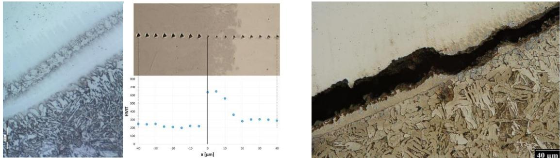
Fig. 2 Path for stress corrosion cracking degradation [4]
