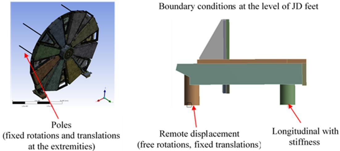
Fig. 3: Simulation model with boundary conditions
