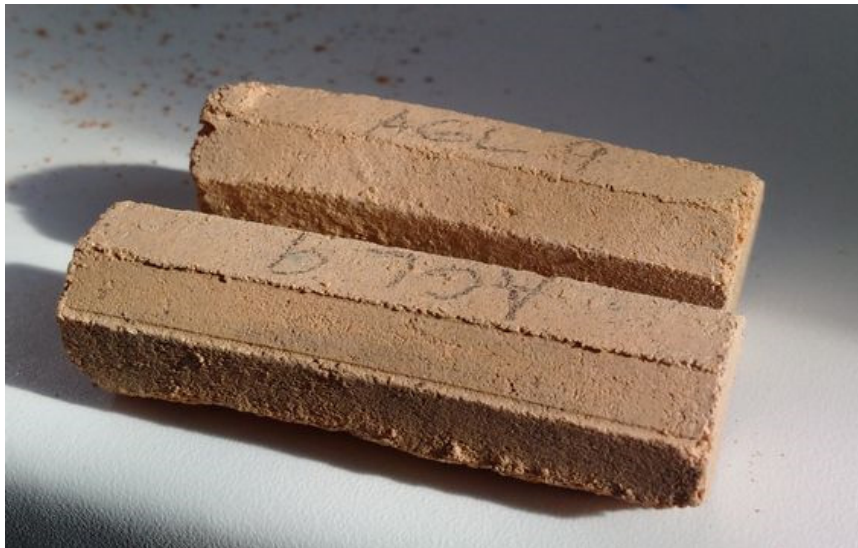
Fig. 1: Specimens for creep and shrinkage tests prepared from Illitic clay.
