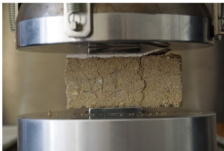
Fig. 4: Specimen for material test prepared from Illitic – kaolinitic clay.
