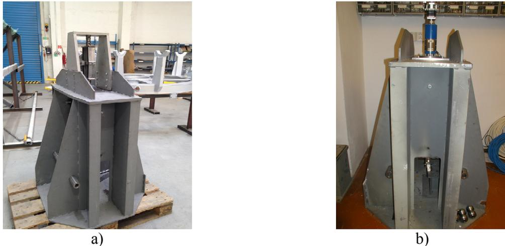
Fig. 4 Stand a) with mechanical reductor, b) without mechanical reductor
