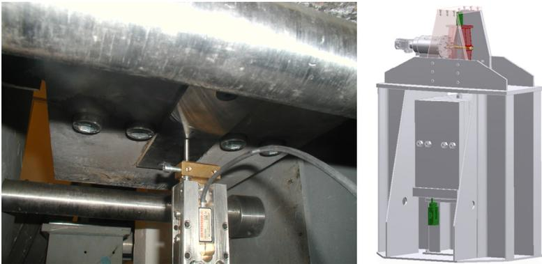
Fig. 7 The displacement sensor located at the bottom part of the stand
