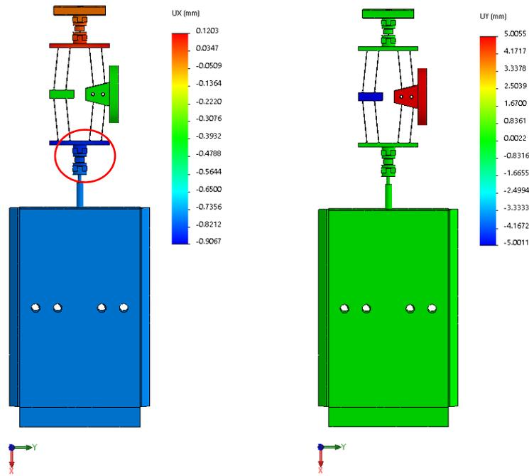
Fig. 2 Displacement fields of points in X and Y direction, respectively
