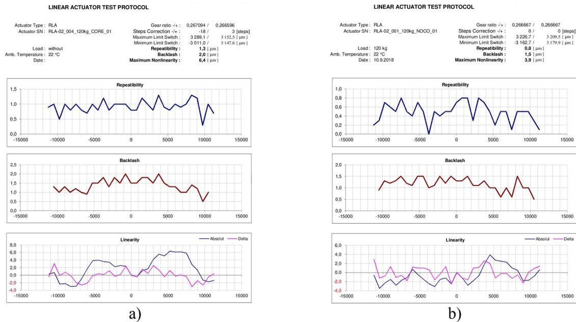
Fig. 8 Test protocol of actuator RLA a) without load, b) with load
