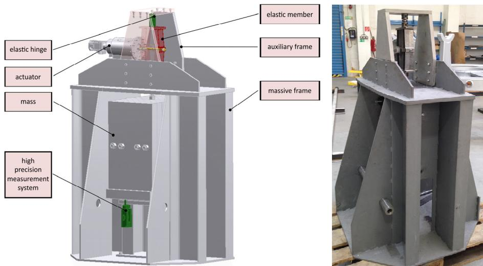
Fig. 1: Numerical and real model of the stand with elastic member and reductor
