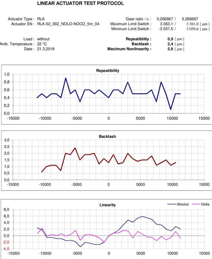
Fig. 6 Linear actuator test protocol without load
