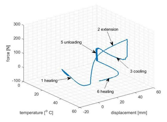
Fig. 2: Cyclic thermo-mechanical loading of thermo-responsive SMP
