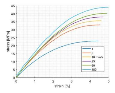
Fig. 4: Tensile tests of Estane with different strain rate
