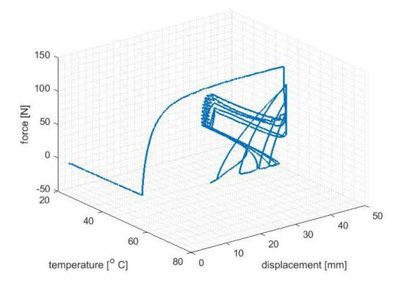
Fig. 7: Result of five cycles Programming - Shape Recovery with the programming temperature  $T_{max} = 57^{\circ}C$  and cooling temperature  $T_{min} = 25^{\circ}C$
