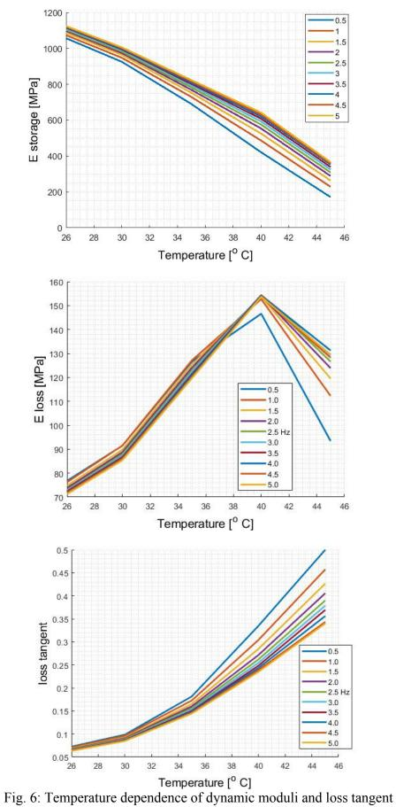
The dynamic moduli and loss tangent as the functions of temperature and frequency are depicted in Fig. 5 and 6. It is seen that the storage modulus E' is rising with the rising frequency and decreases gradually with increasing temperature. The loss modulus E'' and loss tangent have the opposite tendency concerning frequency and they show the rising towards the glass transition temperature.
