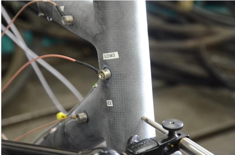
Fig. 7: Location of AE sensors
