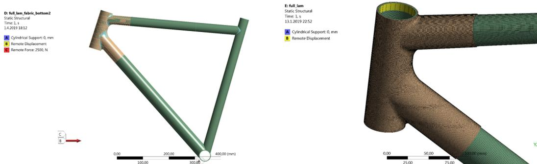
Fig. 9: Geometry of the bike frame model with the detail of the head tube joint shell elements.
