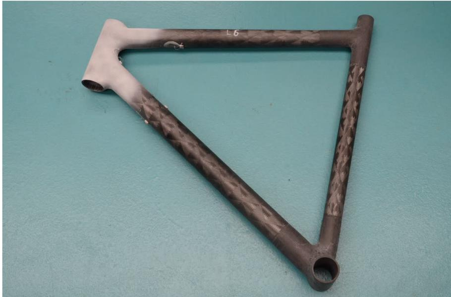
Fig. 1: Simplified composite bicycle frame
