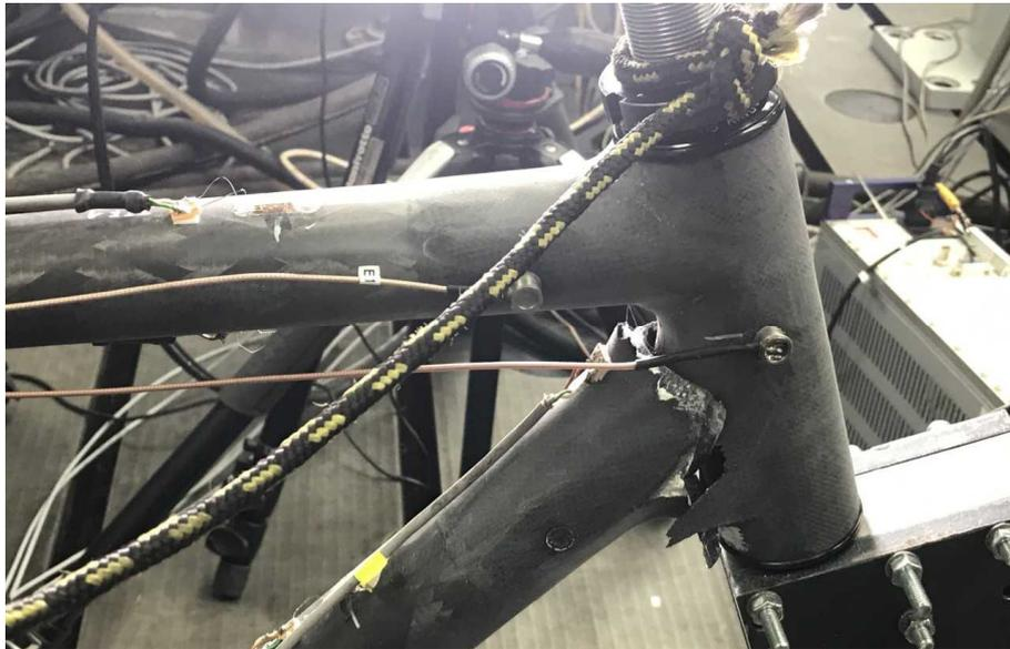
Fig. 12: The down tube-head tube failure during the frame loading.
