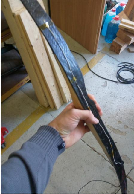
Figure 4: Harness and strain gauge bonded on the recurve bow
