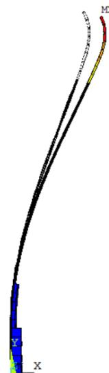
Figure 3: FEM modal shape of the system without the string at 15.80 Hz
