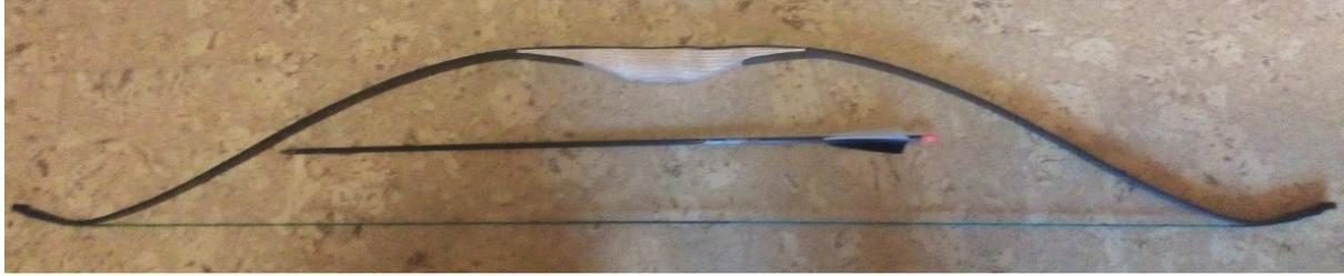
Figure 1: Fabricated recurve bow
