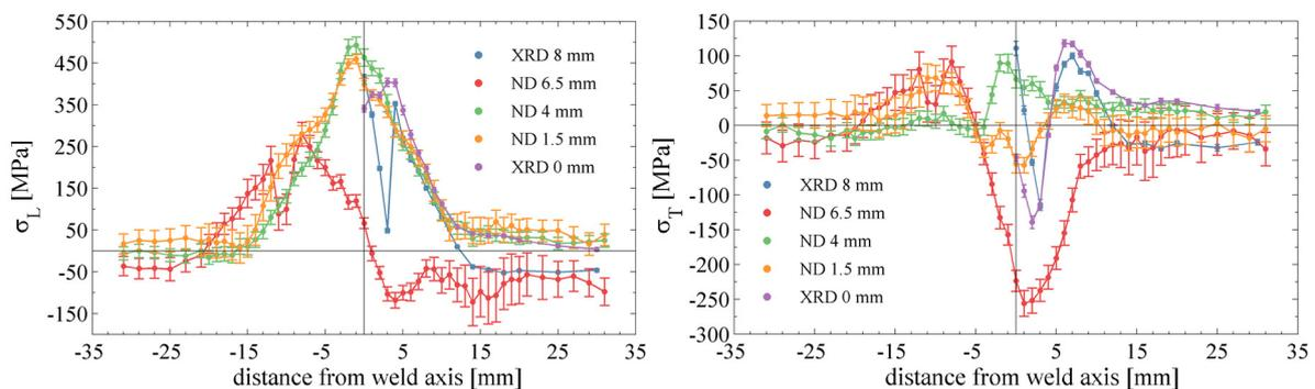
Fig. 5: Longitudinal and transversal RSs for 8 mm thick sample with respect to distance determined across the weld for different depths
