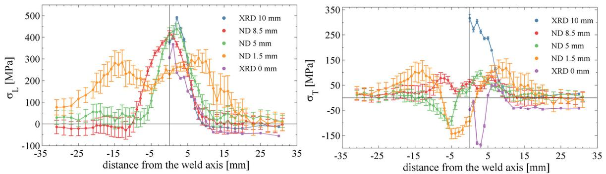
Fig. 4: Longitudinal and transversal RSs for 10 mm thick sample with respect to distance determined across the weld for different depths
