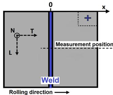
Fig. 1: Scheme of the sample. The cross in the right upper corner denotes the place where the depth profile was measured
