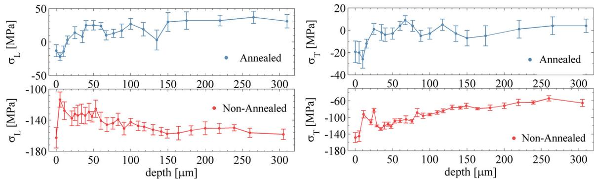
Fig. 2: Longitudinal L (parallel to the weld axis) and transversal T (perpendicular to the weld axis) RSs with respect to depth under the surface
