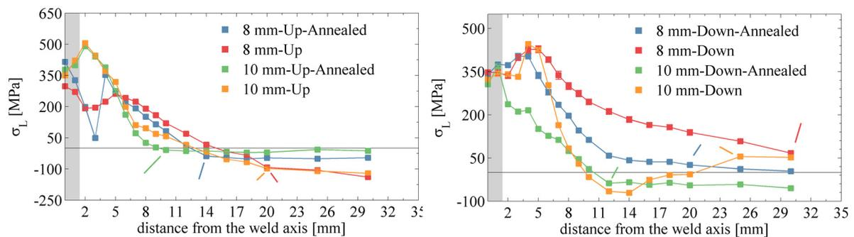
Fig. 3: Longitudinal RSs on “Up” and “Down” side determined for annealed and non-annealed plates
