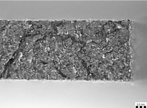
Fig. 8: Fracture surface – specimen C30
