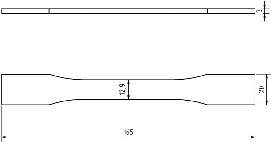
Fig. 1: Specimen used for tension tests
