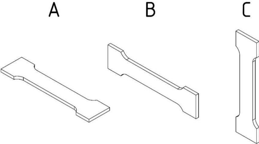
Fig. 2: Orientation of specimens when printed
