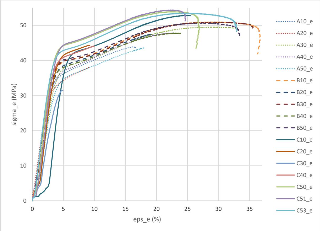
Fig. 3: Tension diagrams of tests performed
