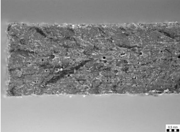
Fig. 5: Fracture surface – specimen A30
