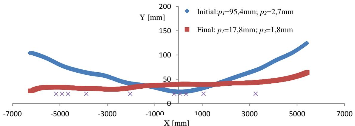
Fig. 6: Shape of the billet before (blue) and after (red) straightening by variant 1
